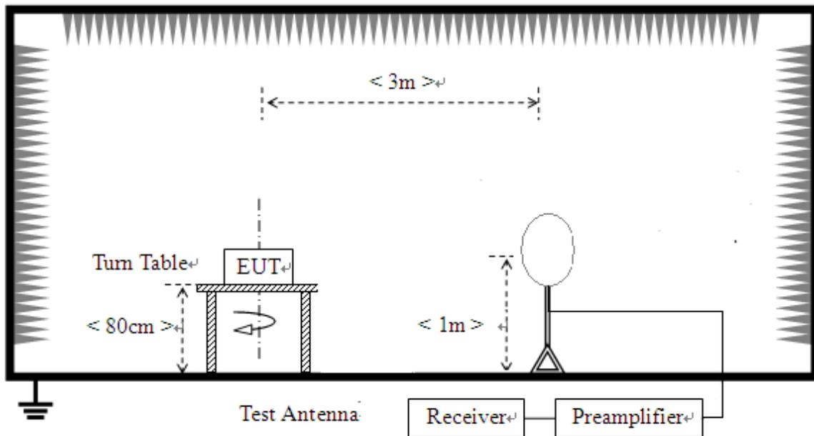
For radiated emissions from 30MHz to 1GHz
