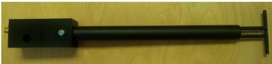
**Figure 1 – MVG COMOSAR Validation Dipole**
