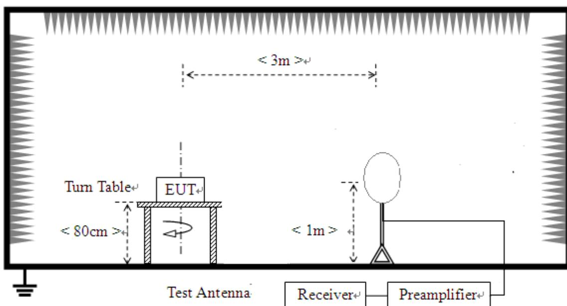
**For radiated emissions from 30MHz to 1GHz**
