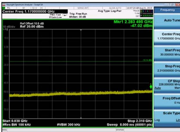
,Plot ,3Transmitter Spurious Emission : 2440,30MHz~2310MHz
