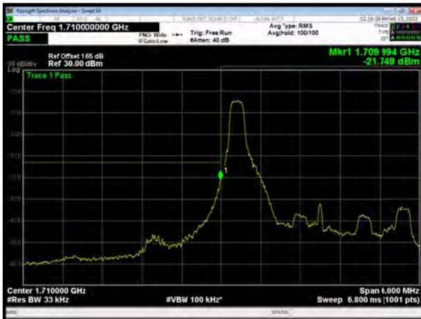
LTE Band 66 16QAM 3MHz CH-High, 1 RB
