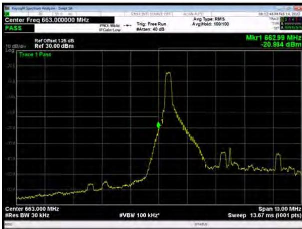
LTE Band 71 16QAM 5MHz CH-High, 1 RB
