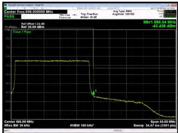
LTE Band 71 16QAM 5MHz CH-Low, 1 RB
