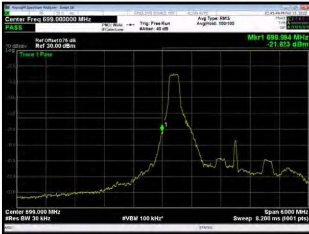
LTE Band 12 64QAM 3MHz CH-High, 1 RB
