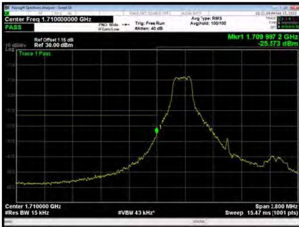
LTE Band 66 64QAM 1.4MHz CH-High, 1 RB
