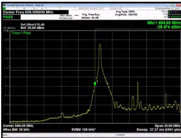
LTE Band 12 64QAM 10MHz CH-High, 1 RB
