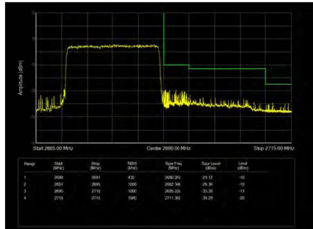
LTE Band 41 64QAM 5MHz CH-Low, 1 RB
