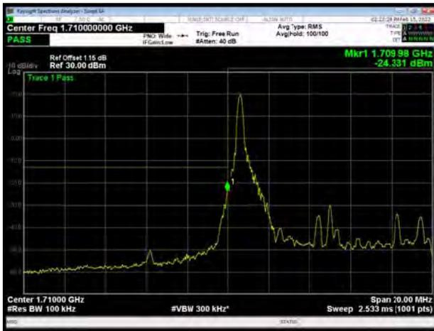
LTE Band 66 64QAM 10MHz CH-High, 1 RB
