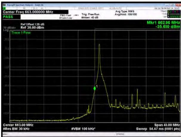
LTE Band 71 16QAM 20MHz CH-High, 1 RB
