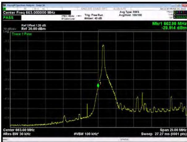
LTE Band 71 16QAM 10MHz CH-High, 1 RB
