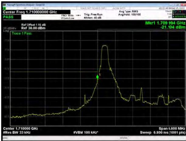
LTE Band 66 64QAM 3MHz CH-High, 1 RB
