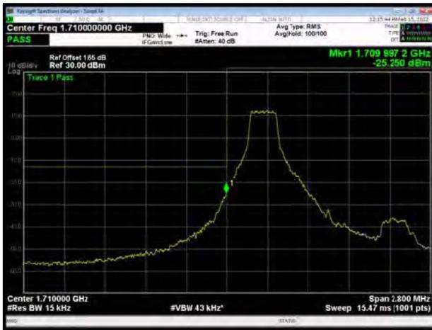
LTE Band 66 16QAM 1.4MHz CH-High, 1 RB
