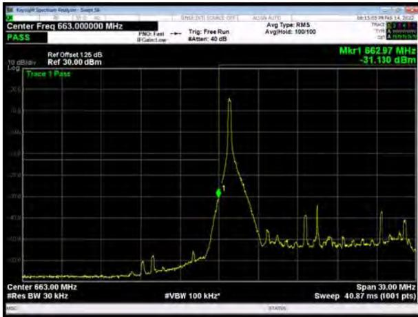
LTE Band 71 16QAM 15MHz CH-High, 1 RB
