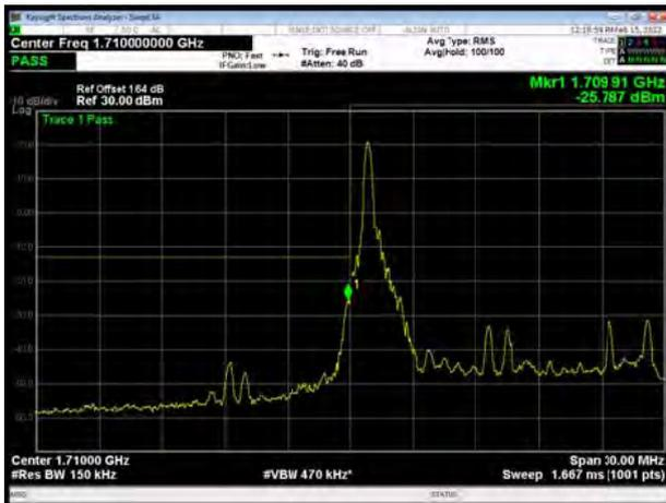
LTE Band 66 16QAM 15MHz CH-High, 1 RB
