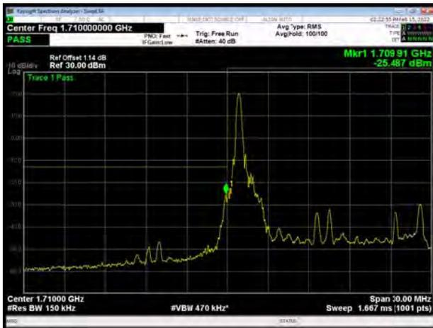
LTE Band 66 64QAM 15MHz CH-High, 1 RB
