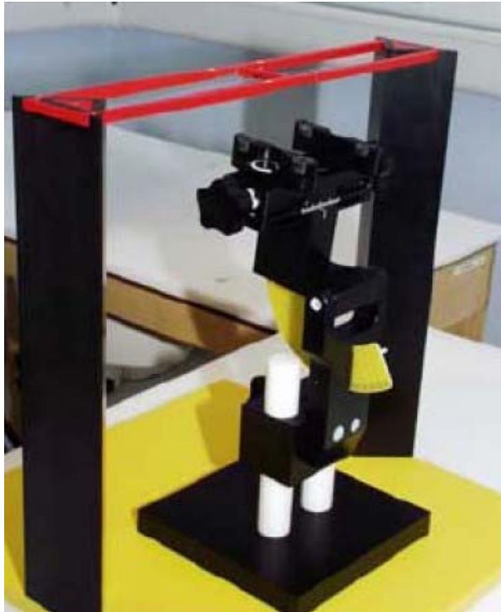
**Figure 7 T-coil Phantom & Device Holder**
