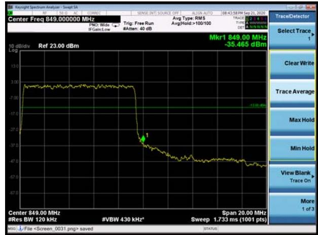
EN-DC\_2A\_n5 16QAM 10MHz CH-Low 1RB
