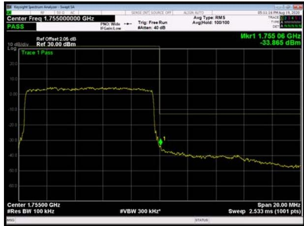
LTE Band 4 16QAM 15MHz CH-Low, 1 RB
