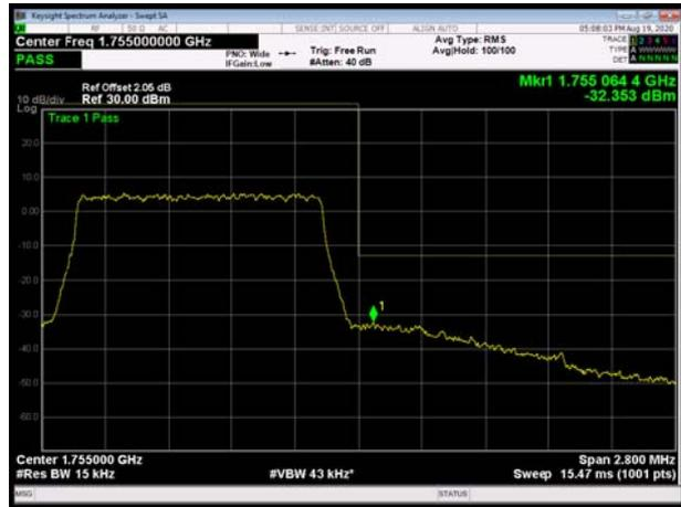
LTE Band 4 16QAM 3MHz CH-Low, 1 RB
