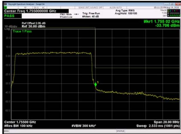
LTE Band 4 64QAM 15MHz CH-Low, 1 RB
