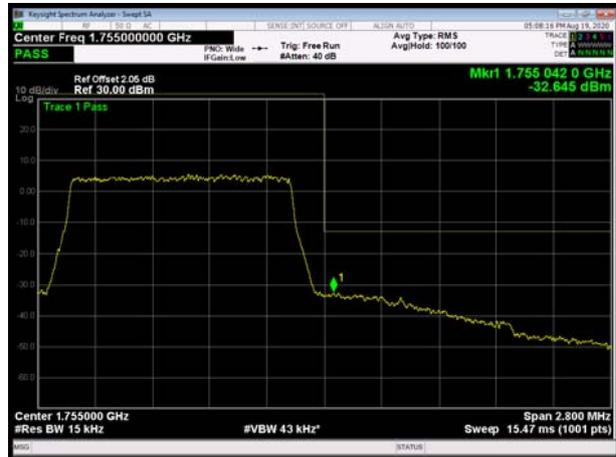
LTE Band 4 64QAM 3MHz CH-Low, 1 RB
