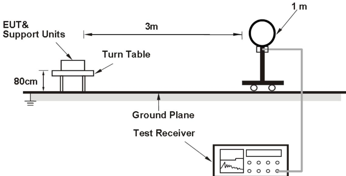
**For Radiated emission 30MHz to 1GHz**
