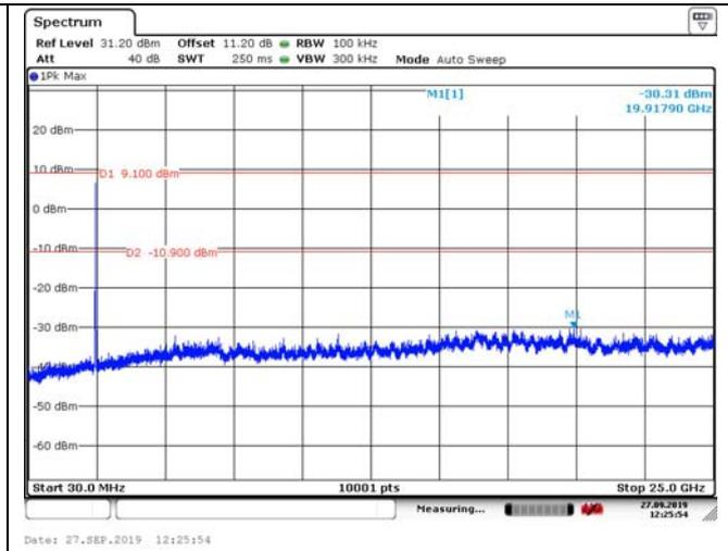
**Band edge measurement (RF Conducted measurement)**
