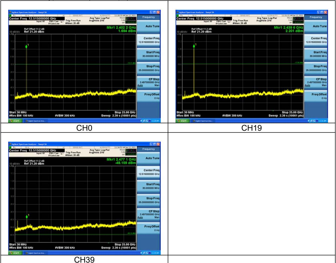
**Band edge measurement (RF Conducted measurement)**
