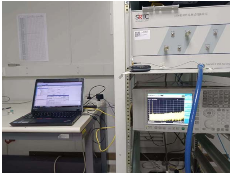
RF Conducted Test setup (BT/WIFI)
