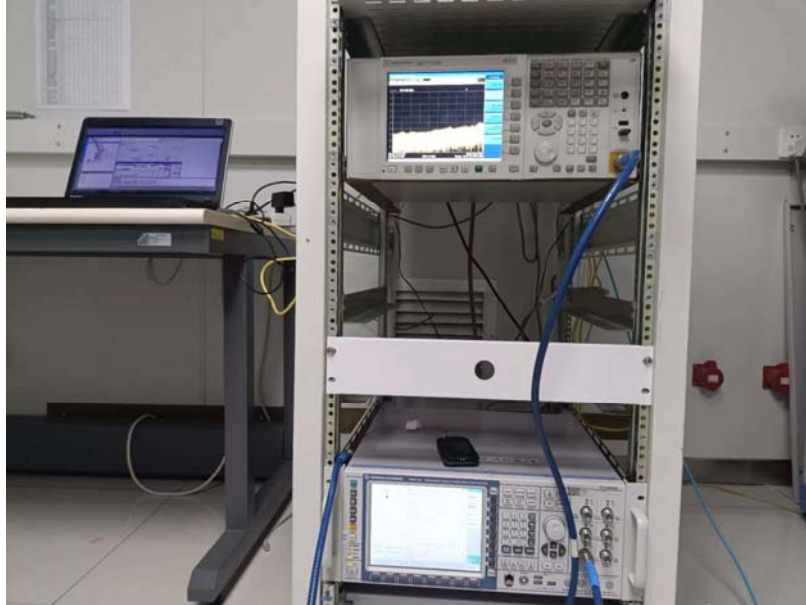
'RF Conducted Test setup (GSM/WCDMA/LTE)
