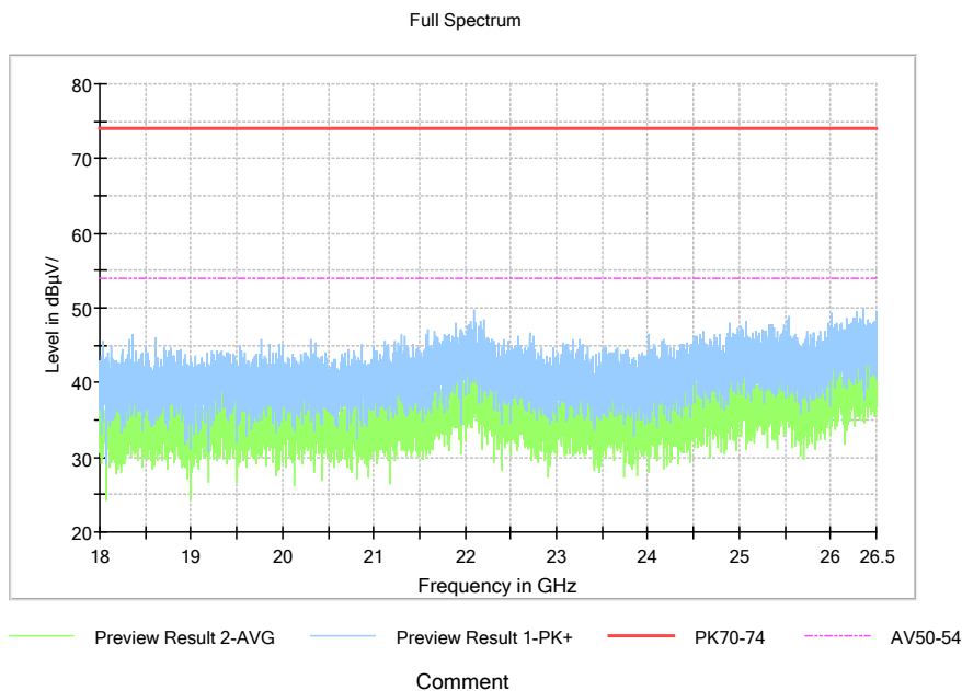
Pic12. Radiated emission (18GHz –26GHz)
