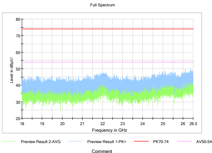
Pic8. Radiated emission (18GHz –26GHz)
