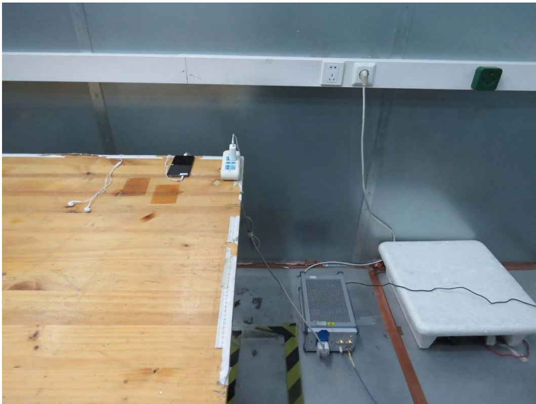
Picture 2 Conducted Emission Test Setup
