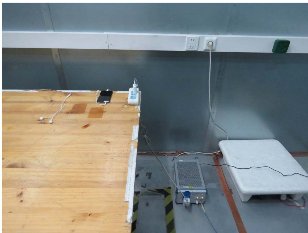
Picture 2 Conducted Emission Test Setup
