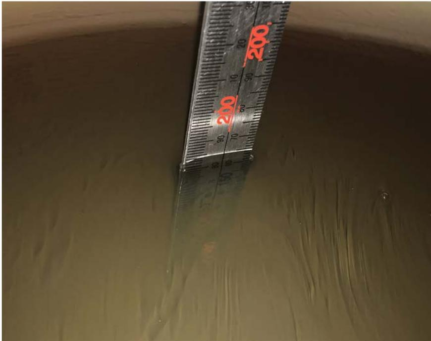
Liquid depth for SAR Measurement
