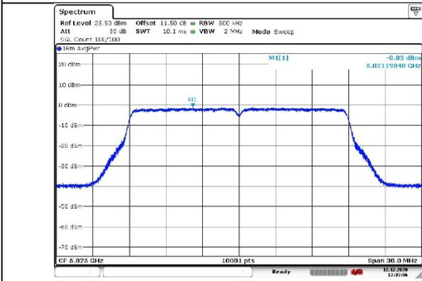
Test Mode: 802.11ac VHT20 Chain1
