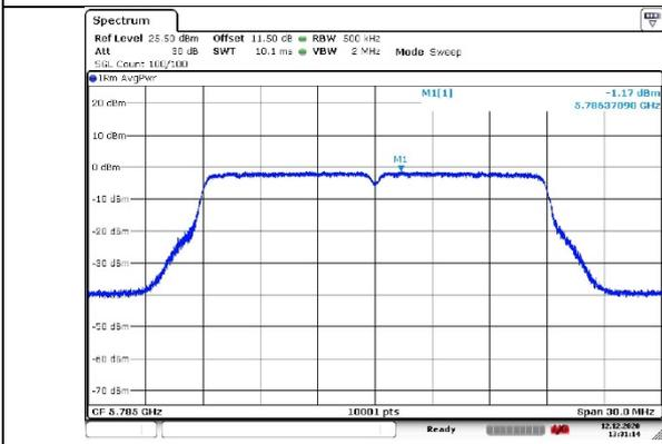
Test Mode: 802.11ac VHT20 Chain1
