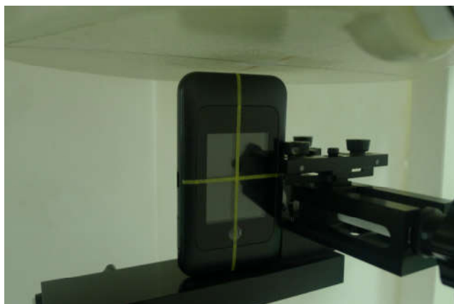
Left Side, Test Separation 10 mm
