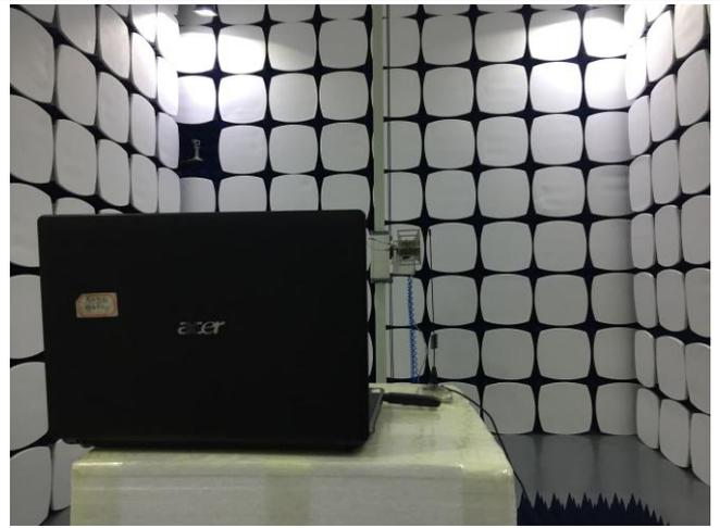
Radiated Spurious Emissions Test Setup Above
