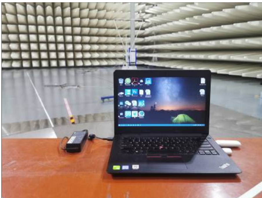
Radiated Emissions Test Setup (30-1000MHz)
