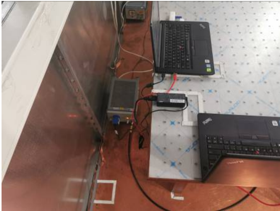
Conducted Emissions Test Setup (with charger)
