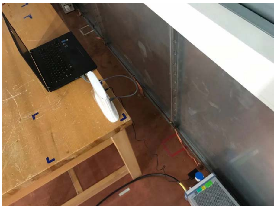
Conducted Emissions Test Setup (with charger)
