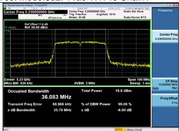
Test Mode:802. 11ac VHT80
