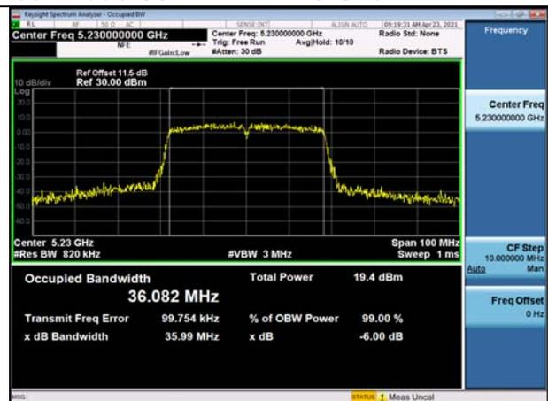
Test Mode:802. 11ac VHT20
