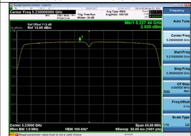
Test Mode:802. 11ac VHT20
