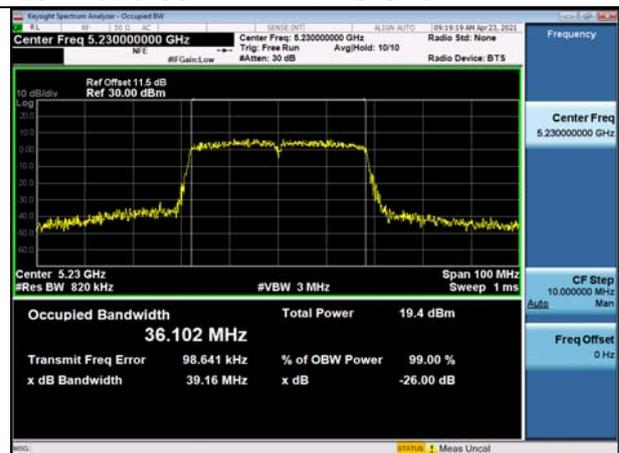
Test Mode:802. 11ac VHT20
