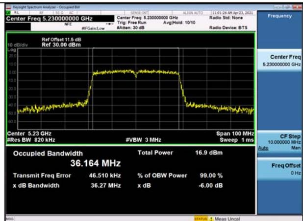
Test Mode:802. 11ac VHT40 Chain1
