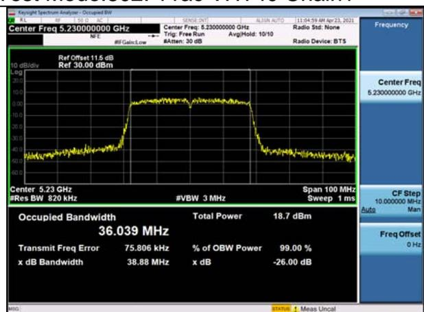
Test Mode:802. 11ac VHT80
