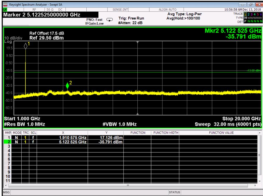
EDGE 850MHz Channel = 251, 30MHz to 1GHz
