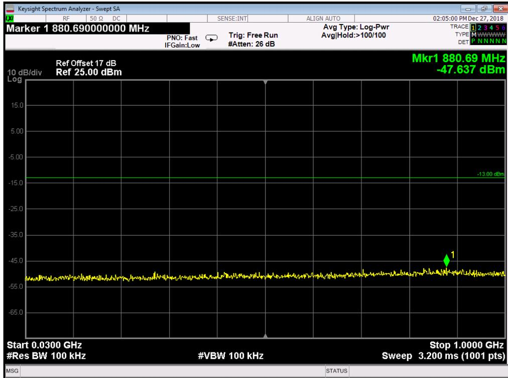
EDGE 1900MHz Channel = 661, 30MHz to 1GHz
