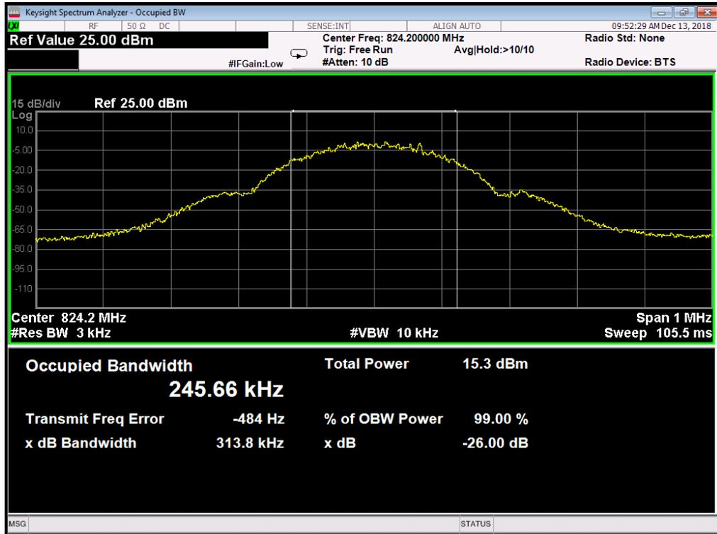
(Plot A1: GSM 850MHz Channel = 128 Occupied bandwidth)
