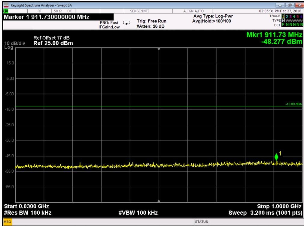
GSM 1900MHz Channel = 810, 30MHz to 1GHz
