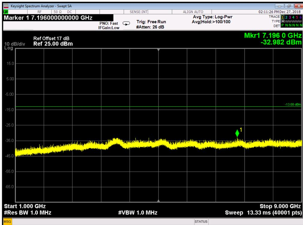
GSM 850MHz Channel = 190, 1GHz to 9GHz
