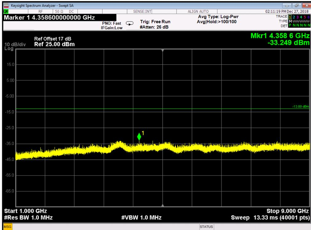
GSM 850MHz Channel = 128, 1GHz to 9GHz
