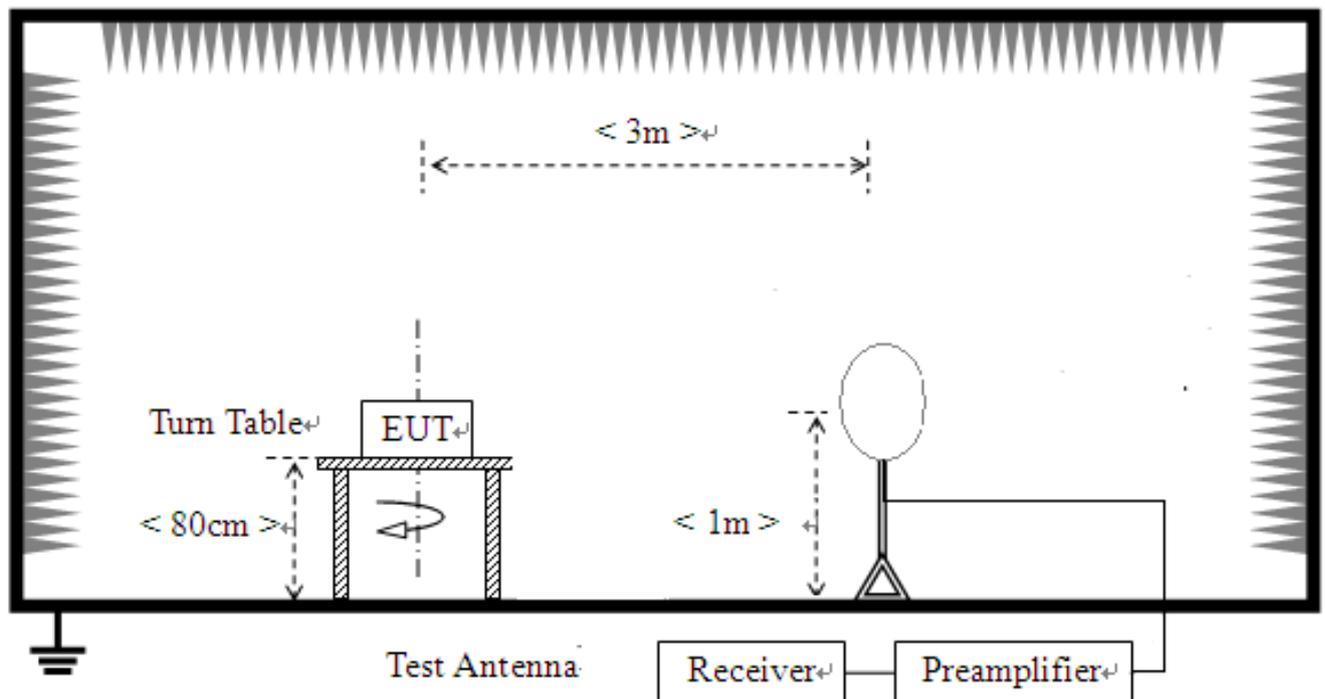
For radiated emissions from 30MHz to 1GHz
