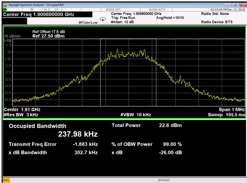
(Plot D3: EDGE 1900MHz Channel = 810 Occupied bandwidth)
