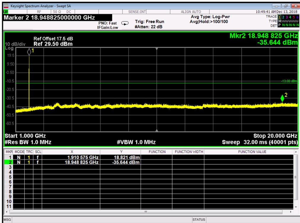
GSM 1900MHz Channel = 810, 1GHz to 20GHz
