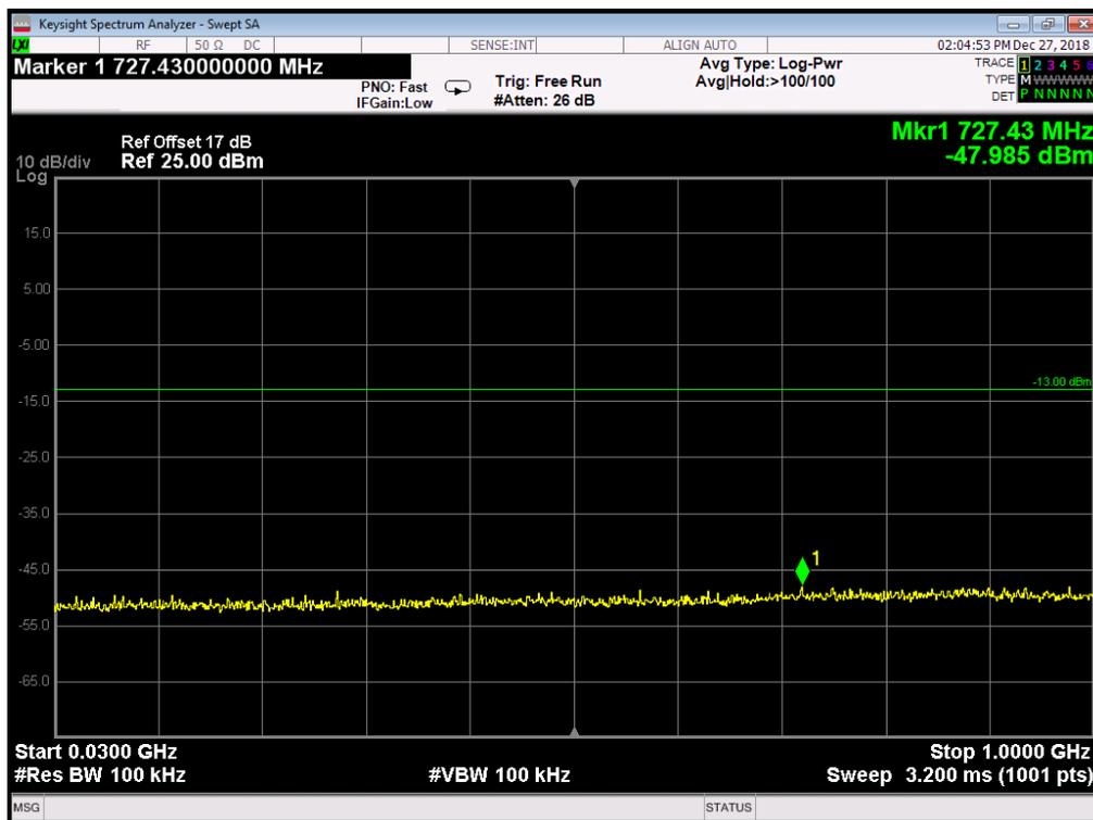
EDGE 850MHz Channel = 128, 1GHz to 9GHz
