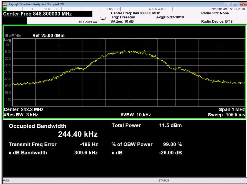
(Plot A3: GSM 850MHz Channel = 251 Occupied bandwidth)
