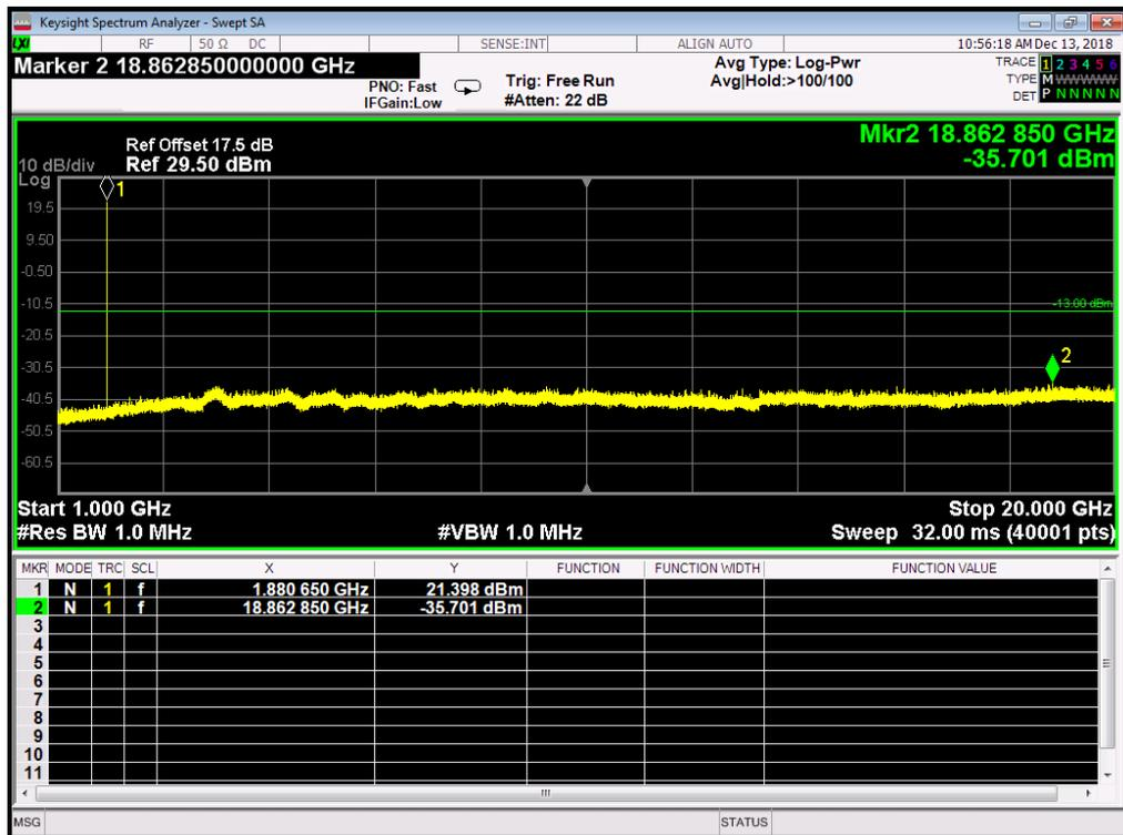
EDGE 1900MHz Channel = 661, 1GHz to 20GHz
