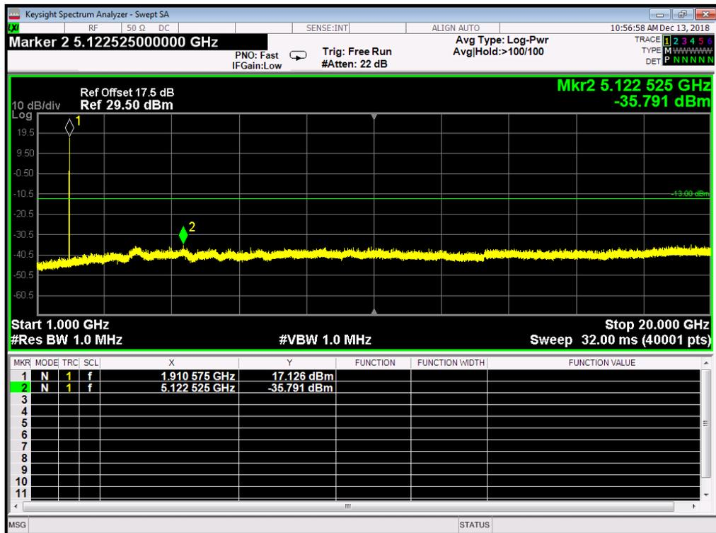
EDGE 1900MHz Channel = 810, 1GHz to 20GHz
