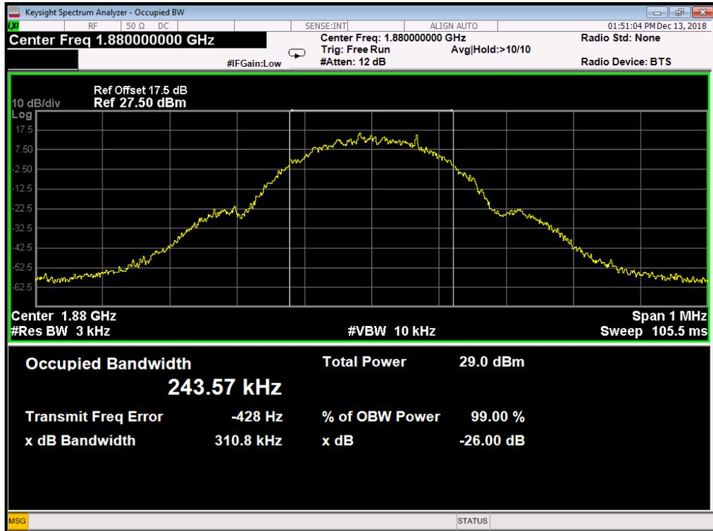
(Plot B2: GSM 1900MHz Channel = 661 Occupied bandwidth)
