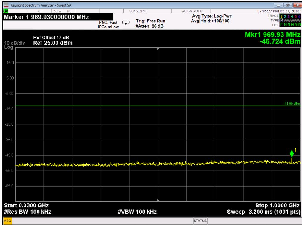
EDGE 1900MHz Channel = 810, 30MHz to 1GHz
