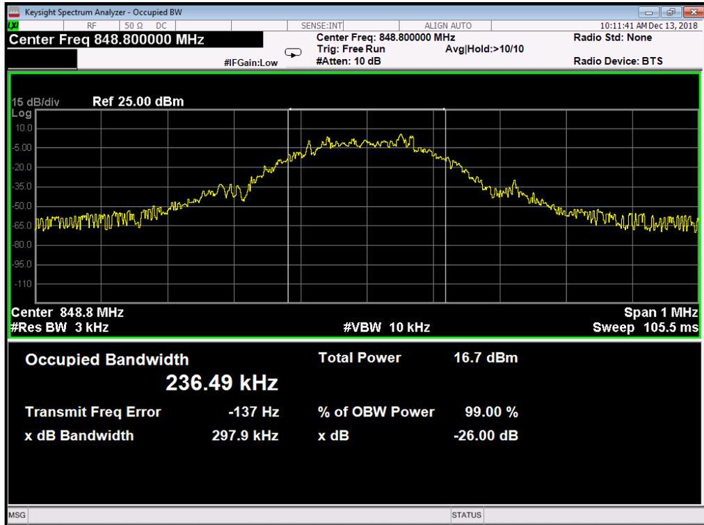
(Plot C3: EDGE 850MHz Channel = 251 Occupied bandwidth)
