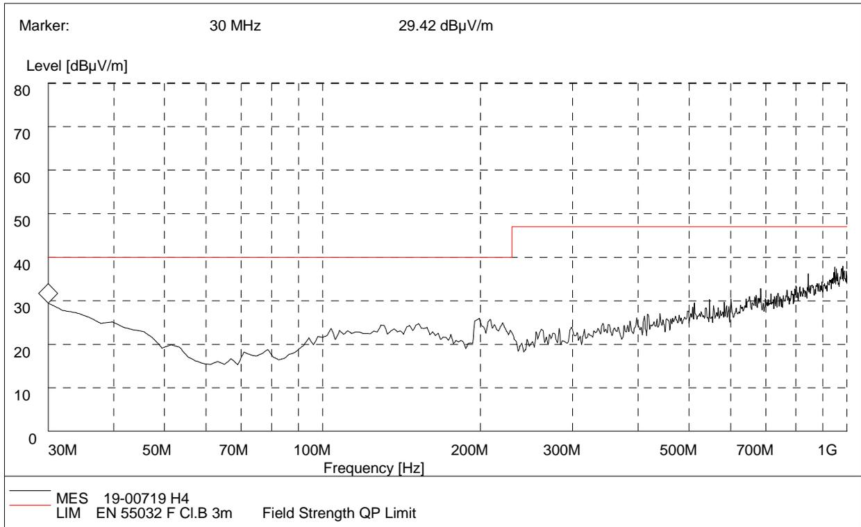
(Plot D: Test Antenna Horizontal 30M - 1G)
