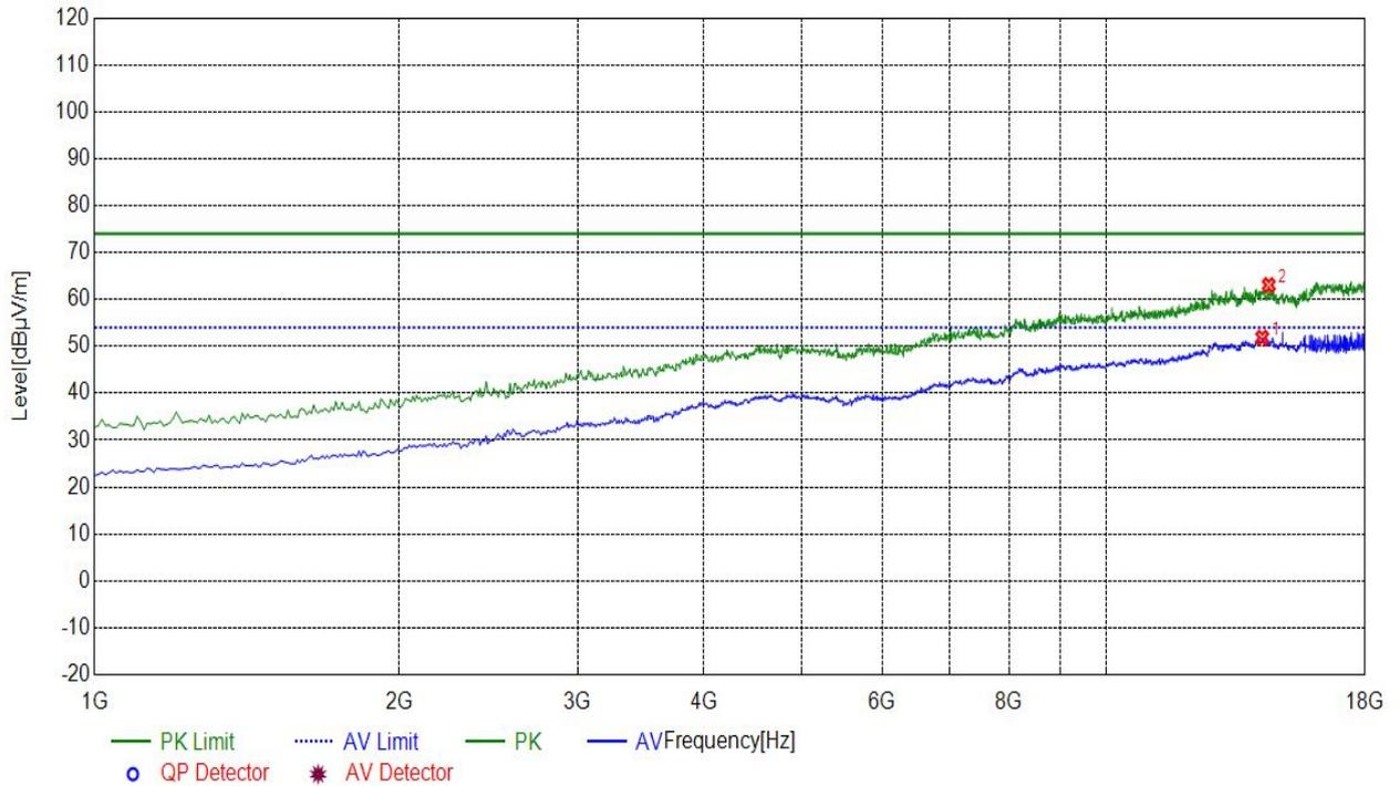
(Plot M: Test Antenna Horizontal 1G – 18G)
