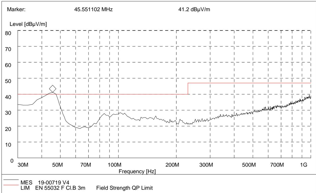
(Plot C: Test Antenna Vertical 30M - 1G)
