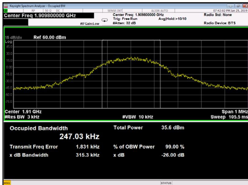
(Plot B3: GSM 1900MHz Channel = 810 Occupied bandwidth)
