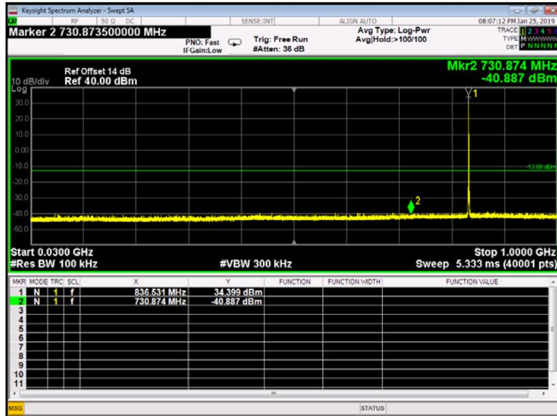
GSM 850MHz Channel = 190, 30MHz to 1GHz
