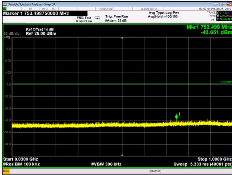
GSM 1900MHz Channel = 512, 30MHz to 1GHz
