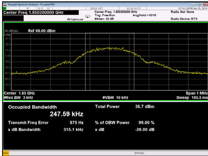
(Plot B1: GSM 1900MHz Channel = 512 Occupied bandwidth)
