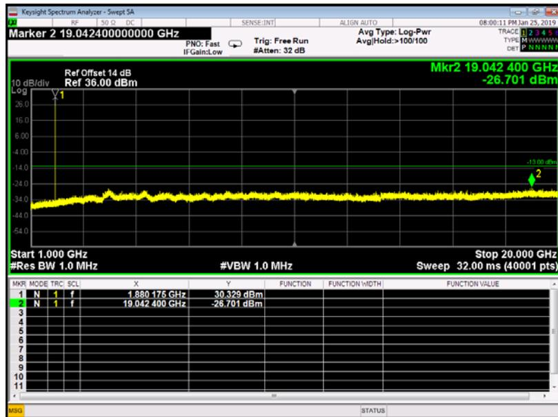
GSM 1900MHz Channel = 661, 1GHz to 20GHz
