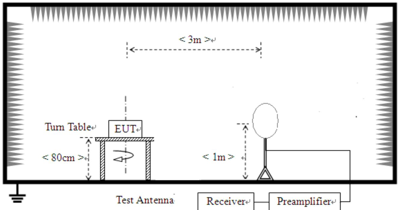
For radiated emissions from 30MHz to 1GHz
