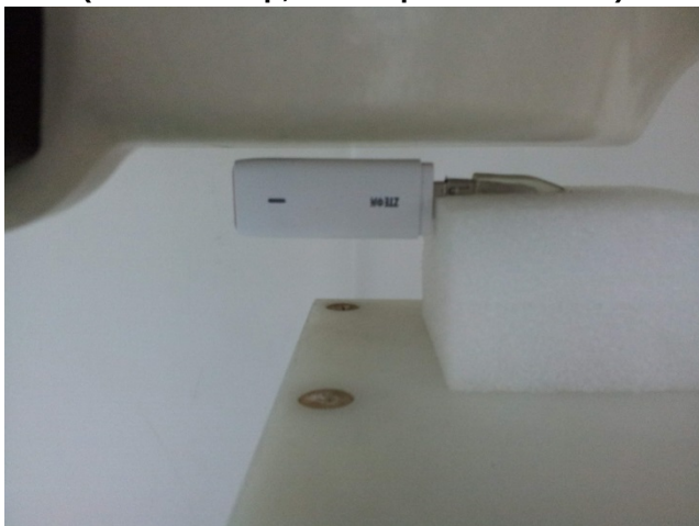
USB Cable Plug-in for USB Configuration 3 (Vertical Front, Test Separation 0.5 cm)
