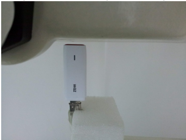
USB Cable Plug-in for USB Configuration 5 (Tip Mode, Test Separation 0.5 cm)
