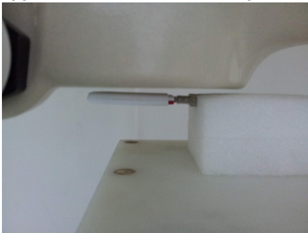
USB Cable Plug-in for USB Configuration 1 (Horizontal Up, Test Separation 0.5 cm)
