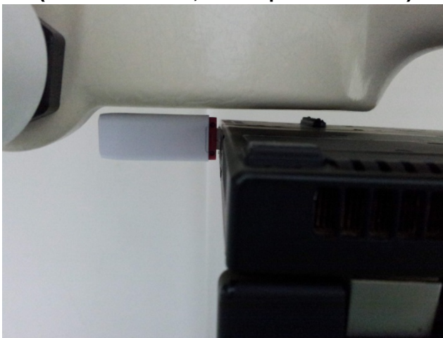
Direct Laptop Plug-in USB Configuration 4 (Vertical Back, Test Separation 0.5 cm)
