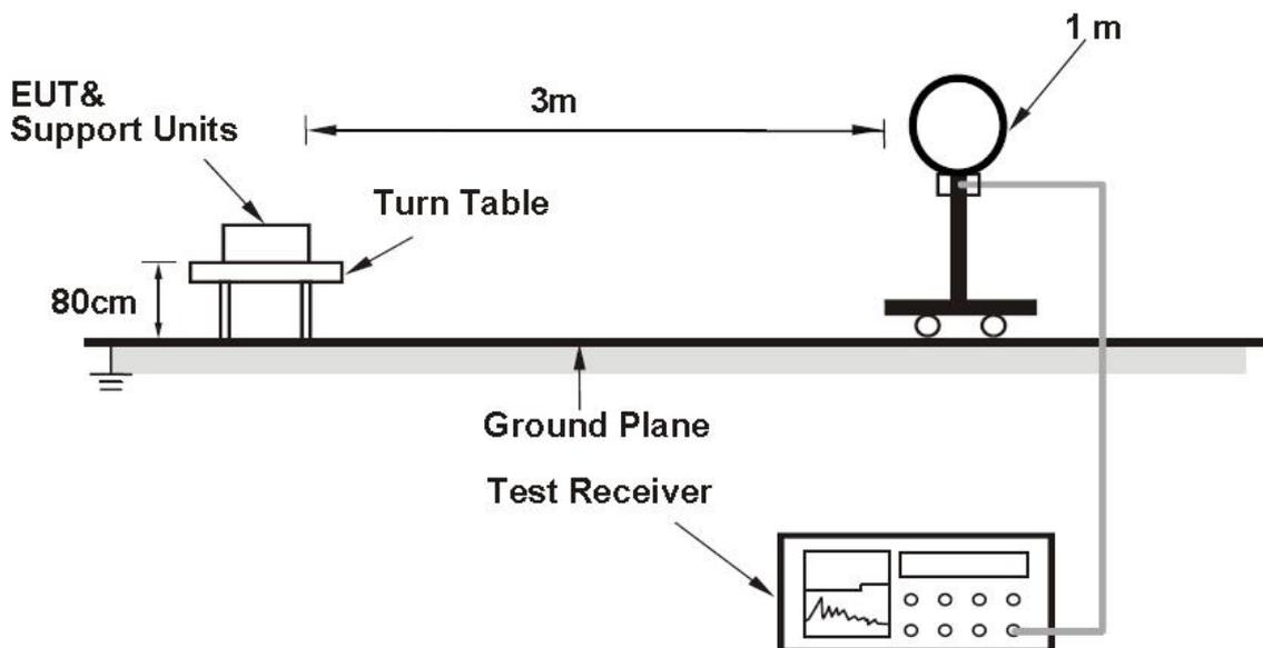
**For Radiated emission 30MHz to 1GHz**
