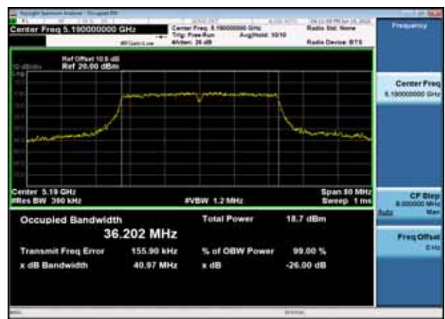
U-NII-1 26dB Bandwidth-802.11ac(40MHz),5190MHz,Ant1
