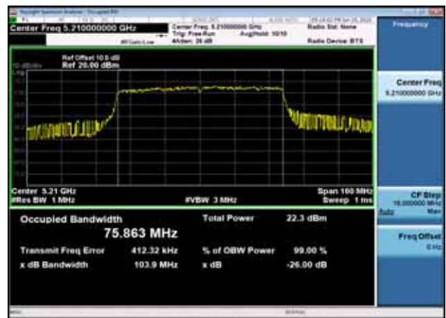
U-NII-2a 26dB Bandwidth-802.11n(20MHz),5260MHz,Ant1
