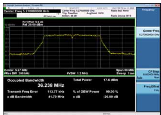
U-NII-2a 26dB Bandwidth-802.11n(40MHz),5270MHz,Ant1
