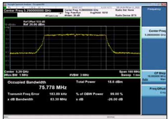
U-NII-2c 26dB Bandwidth-802.11n(20MHz),5500MHz,Ant1
