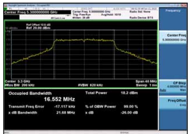
U-NII-2a 26dB Bandwidth-802.11a(20MHz),5300MHz,Ant1
