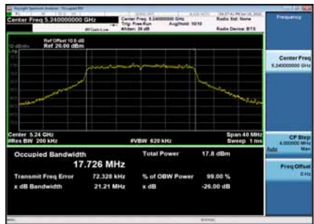
U-NII-1 26dB Bandwidth-802.11ac(40MHz),5190MHz,Ant1
