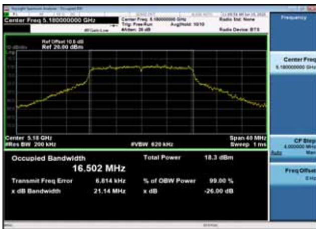
U-NII-1 26dB Bandwidth-802.11a(20MHz) ,5180MHz,Ant0
