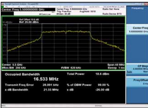
U-NII-2c 26dB Bandwidth-802.11a(20MHz),5600MHz,Ant0
