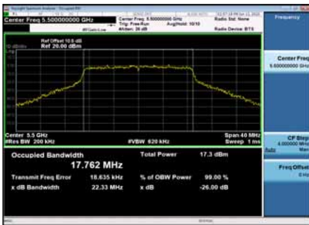
U-NII-2c 26dB Bandwidth-802.11n(20MHz),5600MHz,Ant0
