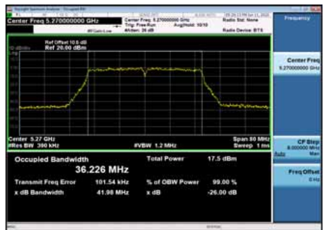
U-NII-2a 26dB Bandwidth-802.11ac(40MHz),5310MHz,Ant1
