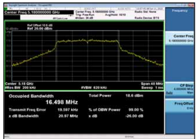
U-NII-1 26dB Bandwidth-802.11a(20MHz) ,5180MHz,Ant1
