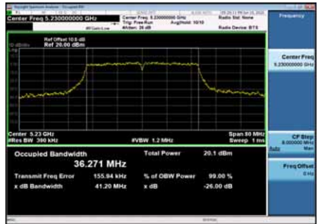
U-NII-1 26dB Bandwidth-802.11a(20MHz) ,5180MHz,Ant1
