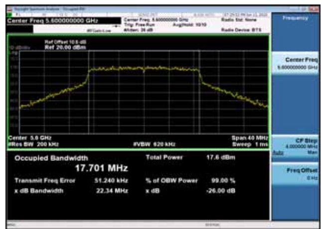
U-NII-2c 26dB Bandwidth-802.11n(20MHz),5600MHz,Ant1
