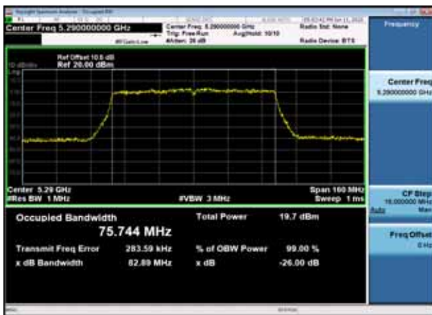
U-NII-2c 26dB Bandwidth-802.11n(20MHz),5500MHz,Ant0
