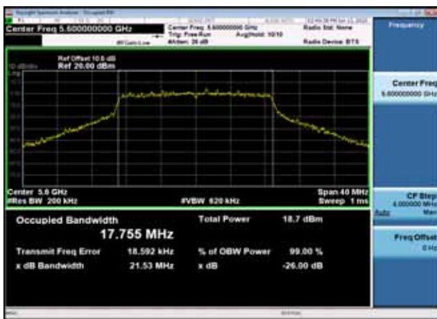
U-NII-2c 26dB Bandwidth-802.11n(20MHz),5600MHz,Ant0
