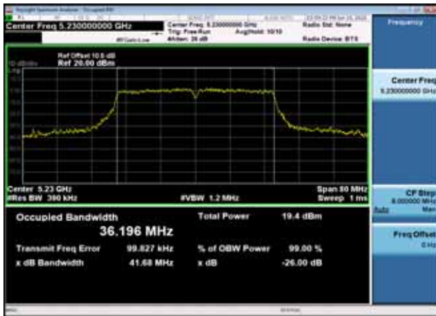
U-NII-1 26dB Bandwidth-802.11a(20MHz) ,5180MHz,Ant0
