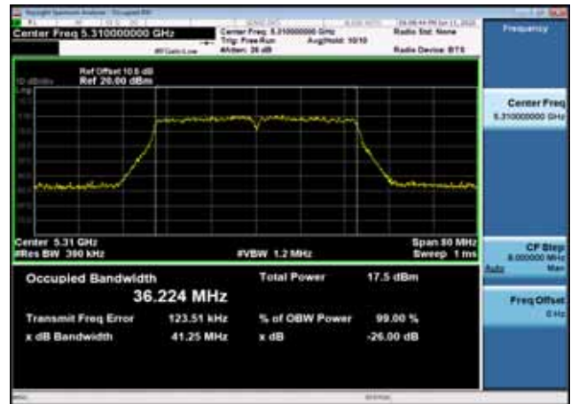
U-NII-2a 26dB Bandwidth-802.11a(20MHz),5260MHz,Ant1
