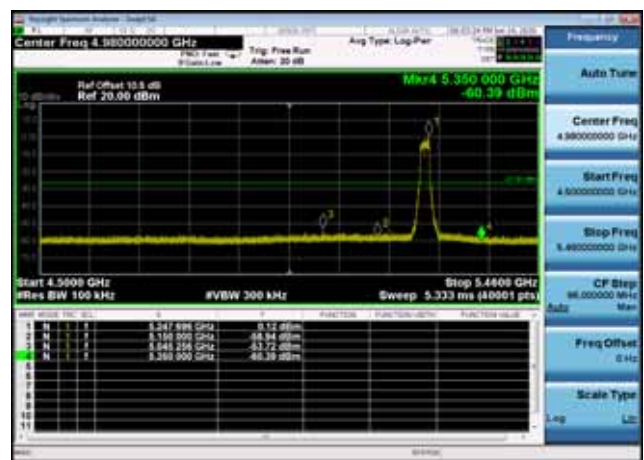
U-NII-1 ,Plot 1,Band Edge-802.11n(20M Hz),5240MHz,Ant1
