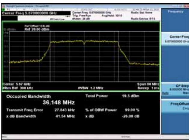
U-NII-2c 26dB Bandwidth-802.11a(20MHz),5500MHz,Ant0
