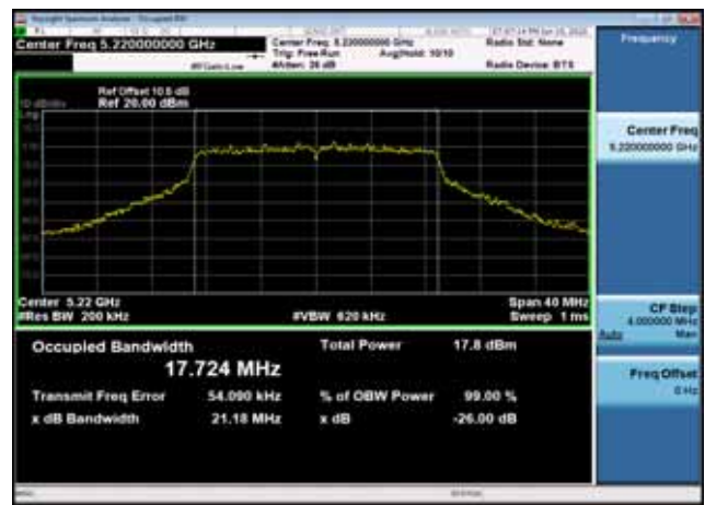
U-NII-1 26dB Bandwidth-802.11ac(20MHz),5240MHz,Ant1
