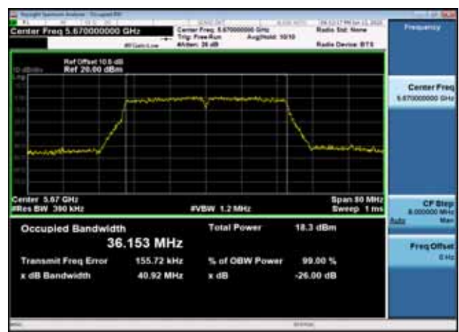
U-NII-2c 26dB Bandwidth-802.11a(20MHz),5500MHz,Ant1
