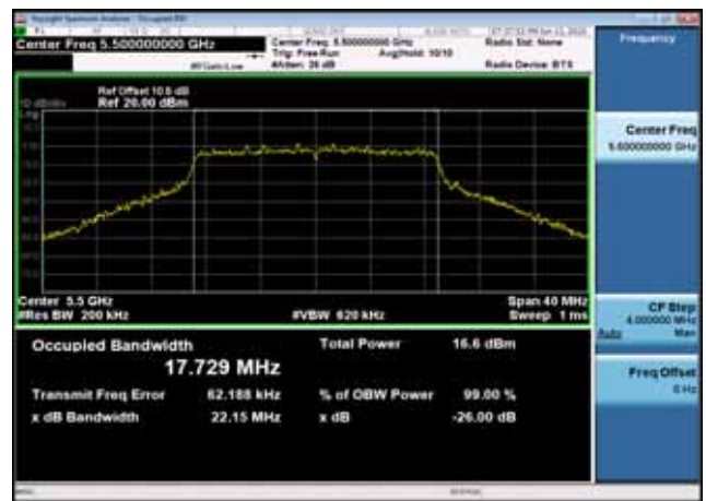
U-NII-2c 26dB Bandwidth-802.11n(20MHz),5600MHz,Ant1
