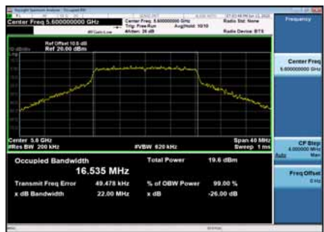
U-NII-2c 26dB Bandwidth-802.11a(20MHz),5600MHz,Ant1
