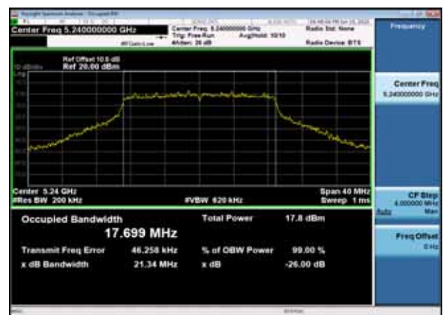
U-NII-1 26dB Bandwidth-802.11n(20MHz) ,5240MHz,Ant1
