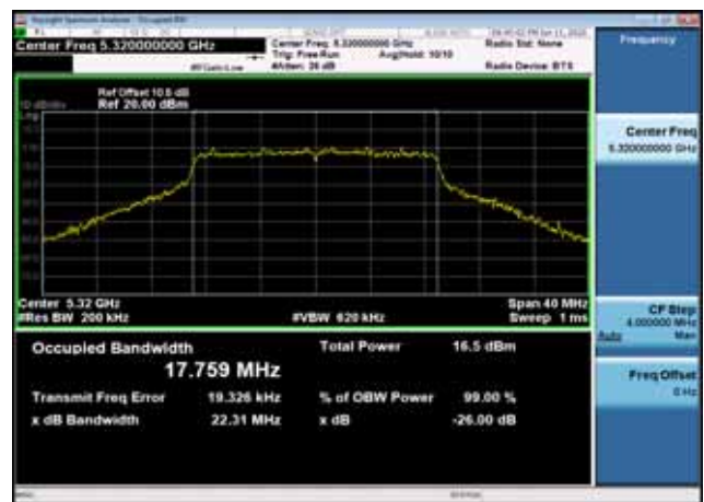
U-NII-2a 26dB Bandwidth-802.11n(40MHz),5270MHz,Ant1
