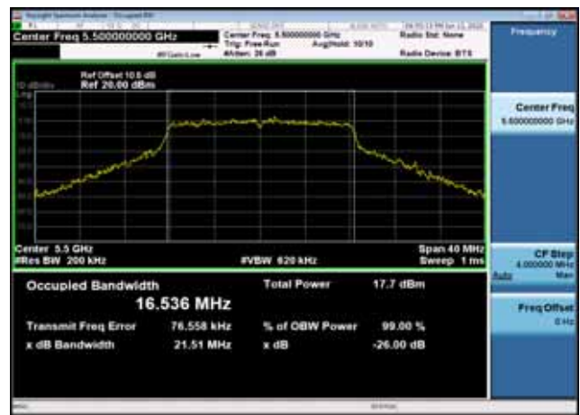
U-NII-2c 26dB Bandwidth-802.11a(20MHz),5600MHz,Ant1
