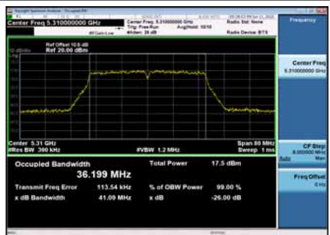
U-NII-2a 26dB Bandwidth-802.11ac(40MHz),5310MHz,Ant1
