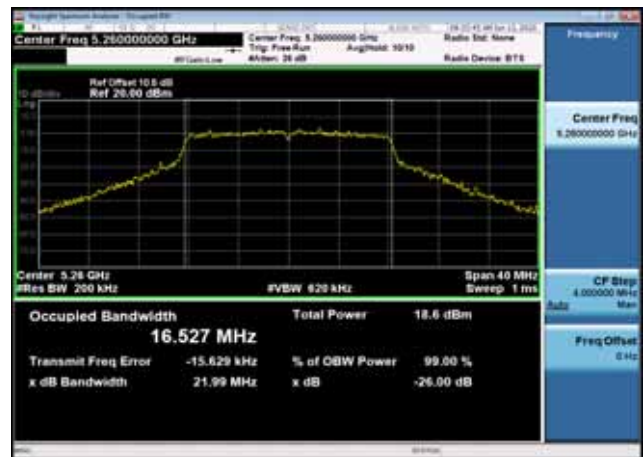
U-NII-2a 26dB Bandwidth-802.11a(20MHz),5300MHz,Ant1
