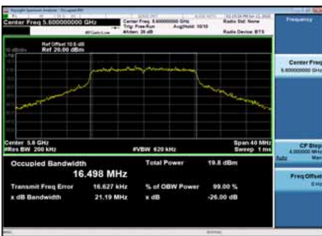
U-NII-2c 26dB Bandwidth-802.11a(20MHz),5600MHz,Ant0
