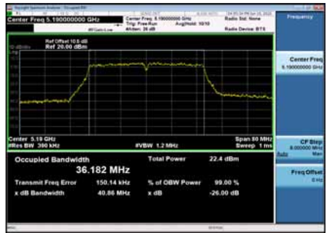
U-NII-1 26dB Bandwidth-802.11n(40MHz) ,5230MHz,Ant1
