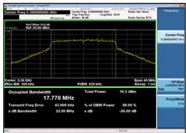
U-NII-2a 26dB Bandwidth-802.11n(20MHz),5260MHz,Ant1
