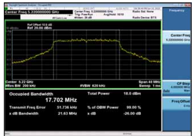
U-NII-1 26dB Bandwidth-802.11n(20MHz) ,5240MHz,Ant1
