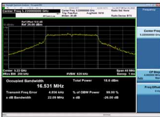
U-NII-1 26dB Bandwidth-802.11a(20MHz) ,5240MHz,Ant0
