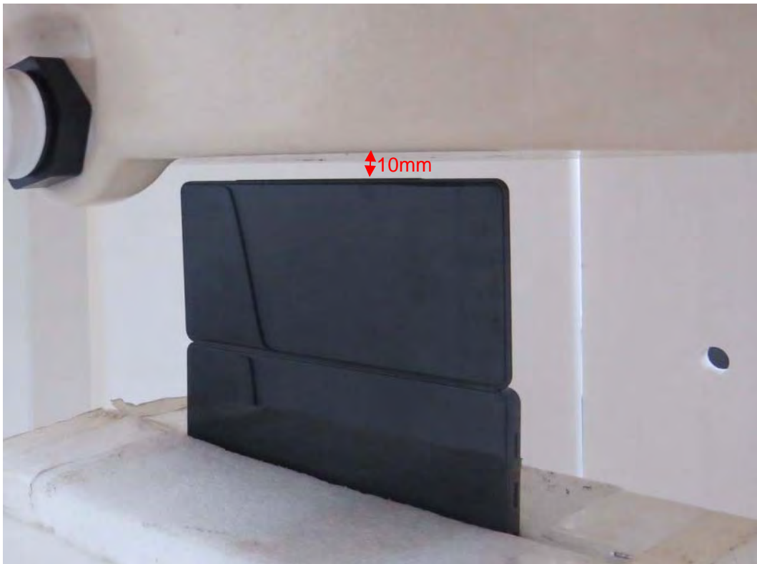
Picture 29: Right Side, the distance from handset to the bottom of the Phantom is 10mm For Double Screen Mode
