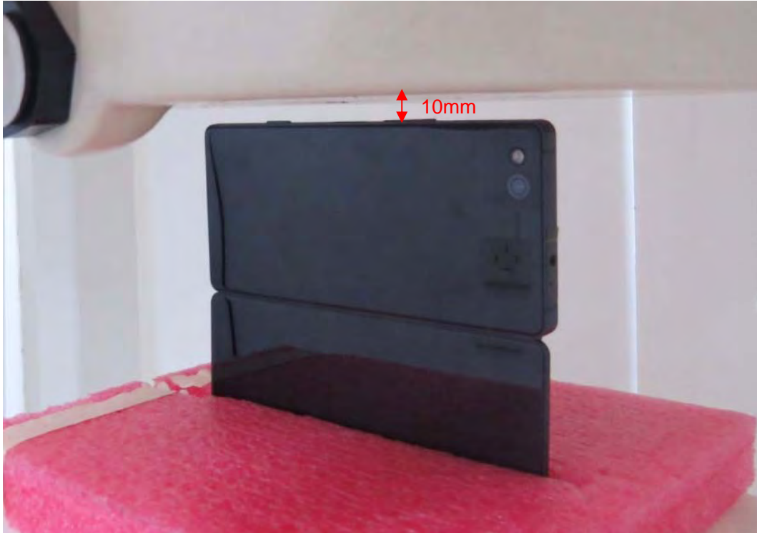
Picture 28: Left Side, the distance from handset to the bottom of the Phantom is 10mm For Double Screen Mode
