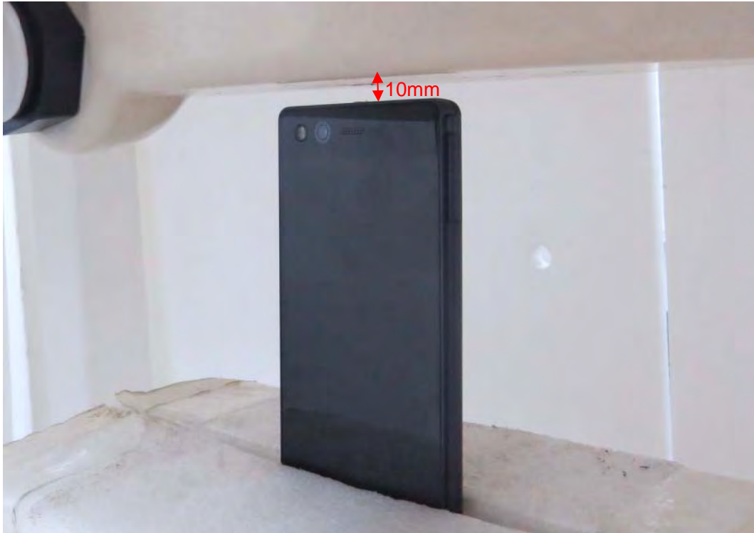
Picture 24: Top Side, the distance from handset to the bottom of the Phantom is 10mm For Single Screen Mode
