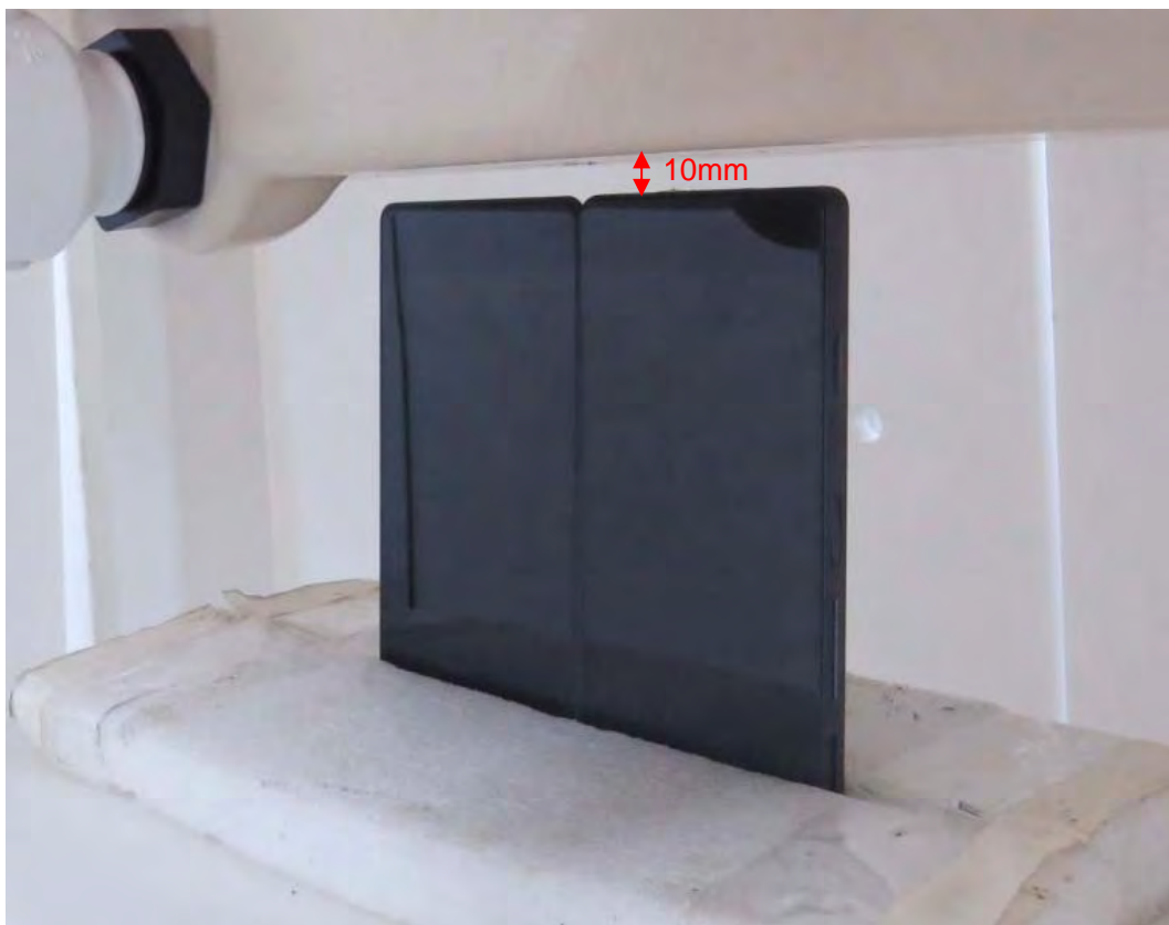
Picture 31: Bottom Side, the distance from handset to the bottom of the Phantom is 10mm For Double Screen Mode
