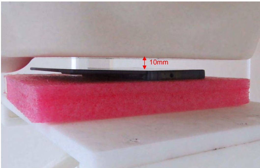
Picture 27: Front Side, the distance from handset to the bottom of the Phantom is 10mm For Double Screen Mode
