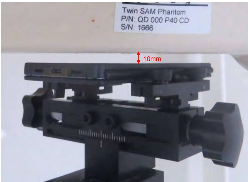
Picture 21: Front Side, the distance from handset to the bottom of the Phantom is 10mm For Single Screen Mode
