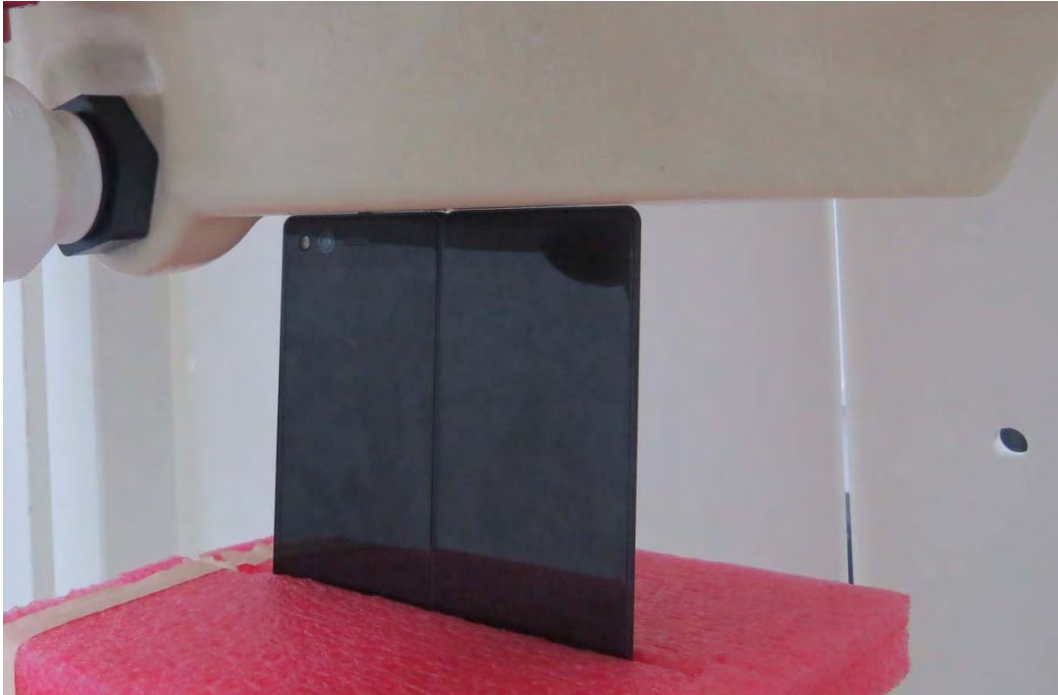
Picture 38: Top Side, the distance from handset to the bottom of the Phantom is 0mm For Double Screen Mode
