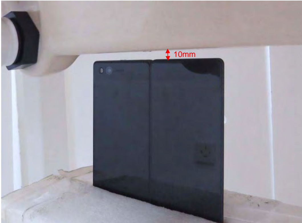
Picture 30: Top Side, the distance from handset to the bottom of the Phantom is 10mm For Double Screen Mode
