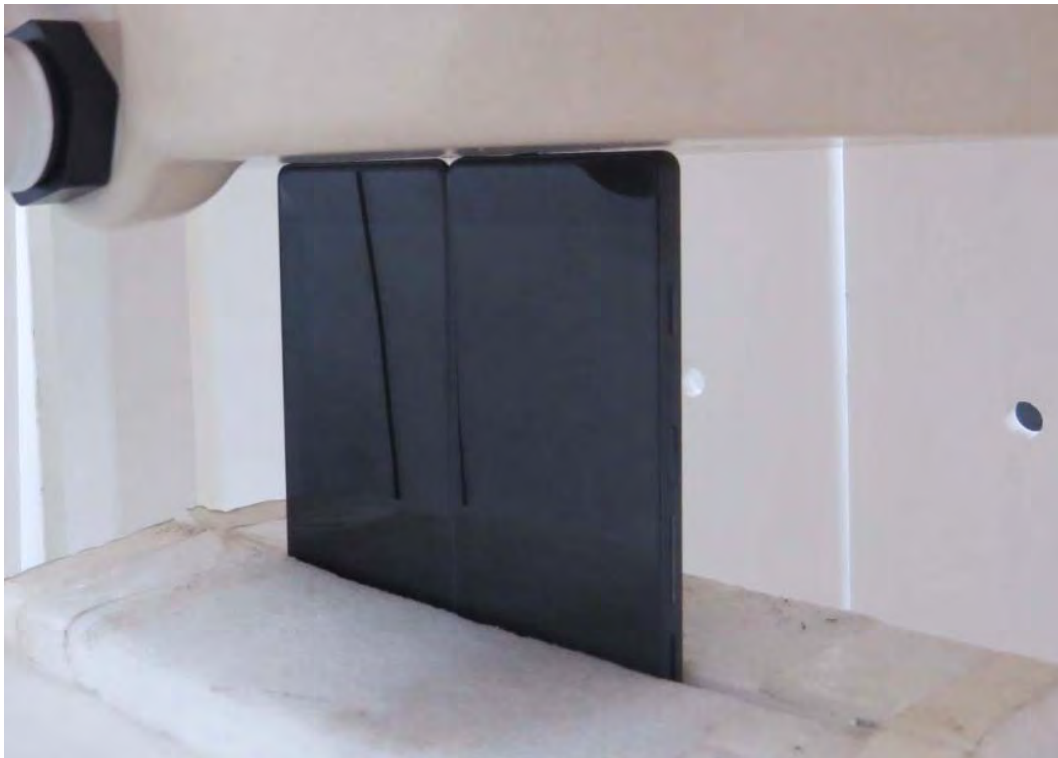
Picture 39: Bottom Side, the distance from handset to the bottom of the Phantom is 0mm For Double Screen Mode
