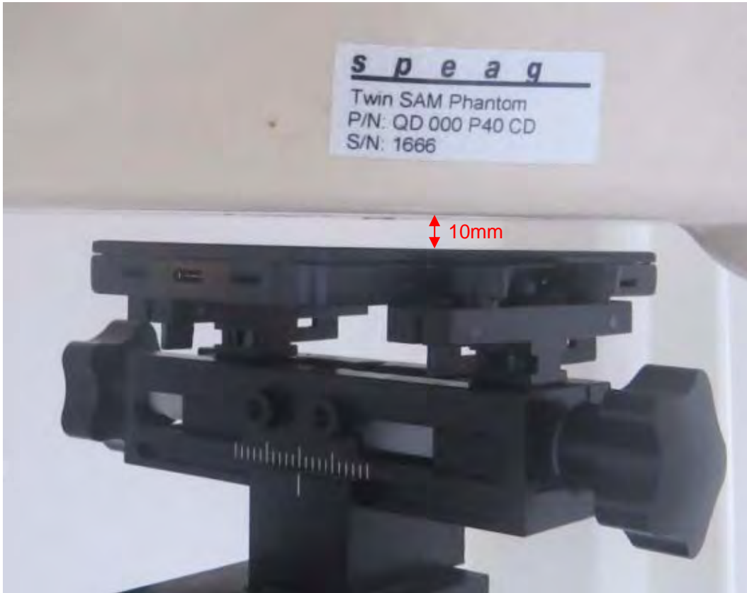
Picture 20: Back Side, the distance from handset to the bottom of the Phantom is 10mm For Single Screen Mode
