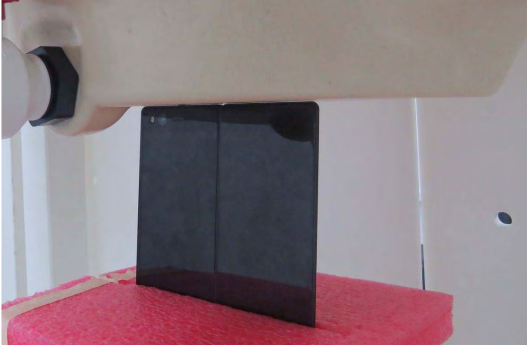
Picture 34: Top Side, the distance from handset to the bottom of the Phantom is 0mm For Double Screen Mode
