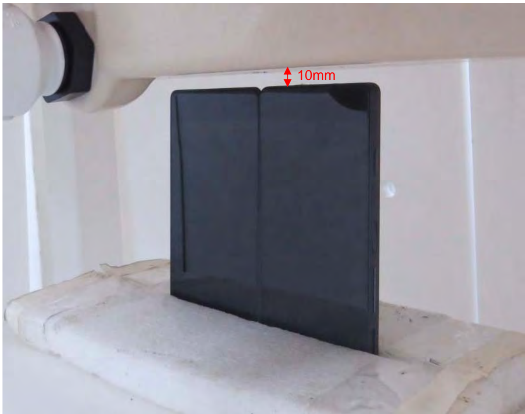
Picture 27: Bottom Side, the distance from handset to the bottom of the Phantom is 10mm For Double Screen Mode
