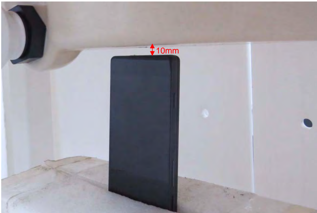
Picture 21: Bottom Side, the distance from handset to the bottom of the Phantom is 10mm For Single Screen Mode
