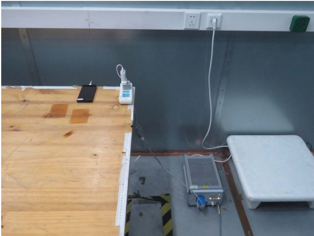
Picture 3 Conducted Emission Test Setup
