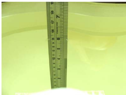
Fig 6.1 Photo of Liquid Height for Head SAR
