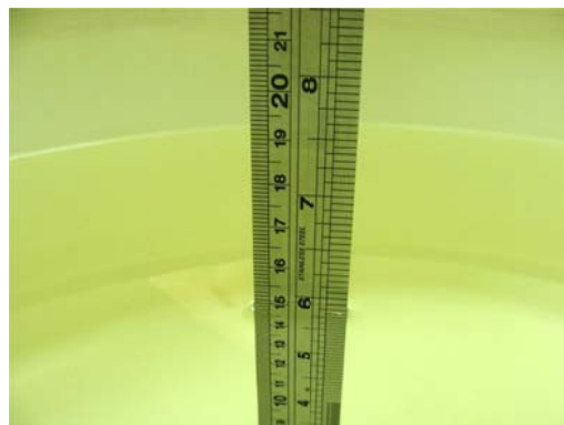
Fig 6.2 Photo of Liquid Height for Body SAR
