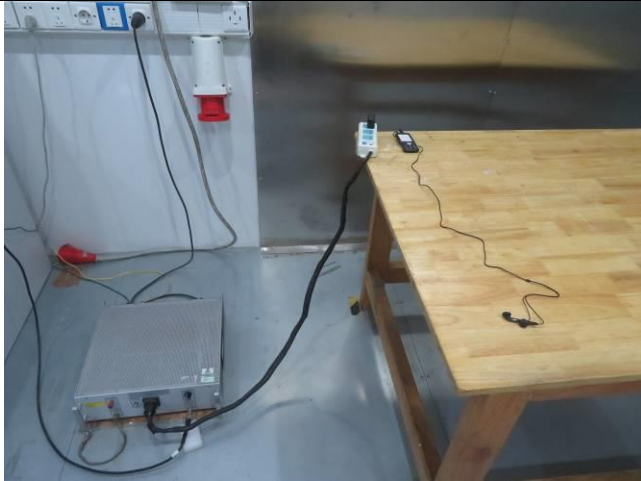
Conducted Emissions Test Setup Front View
