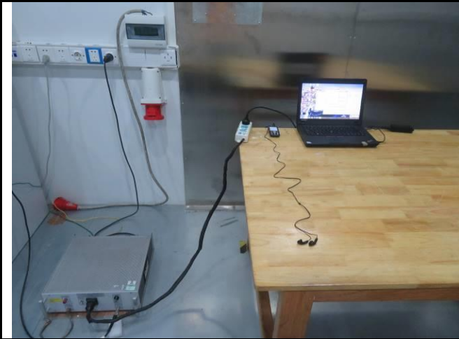
Conducted Emissions Test Setup – Front View
