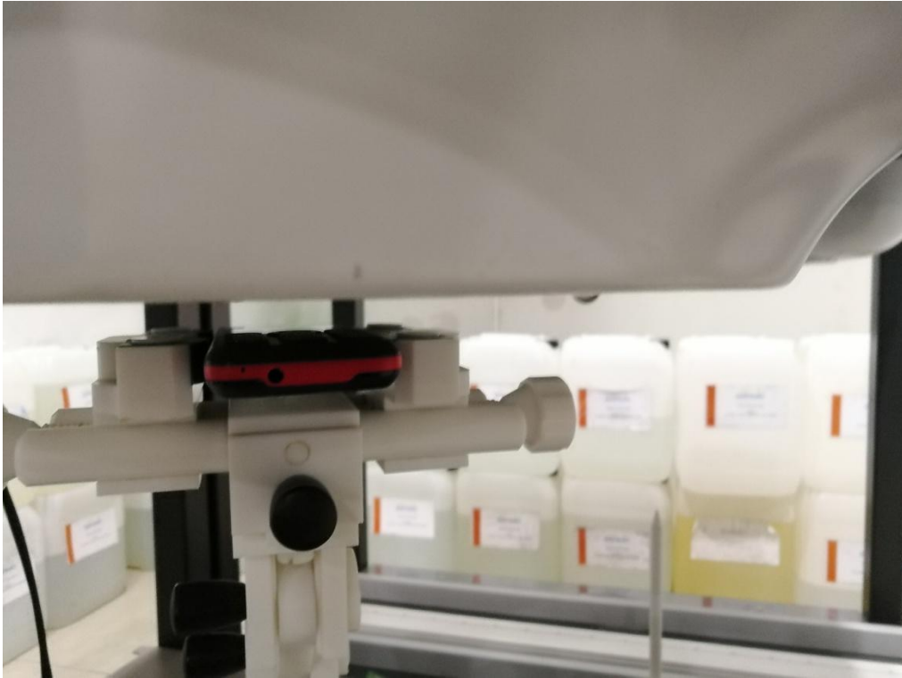
Body Front side(separation distance is 10mm)
