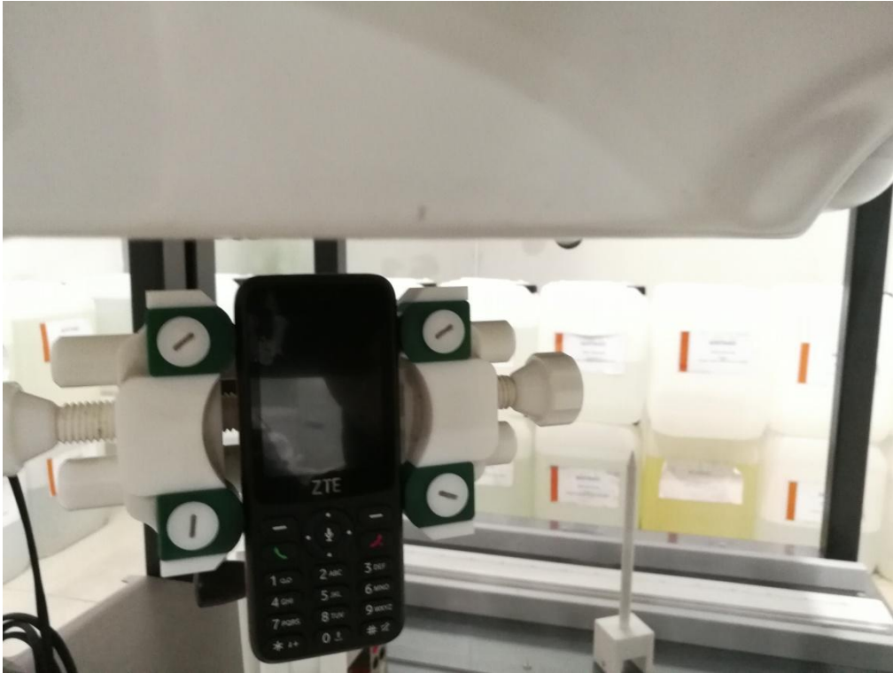
Body Top side(separation distance is 10mm)
