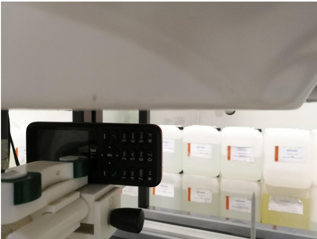
Body Right side(separation distance is 10mm)
