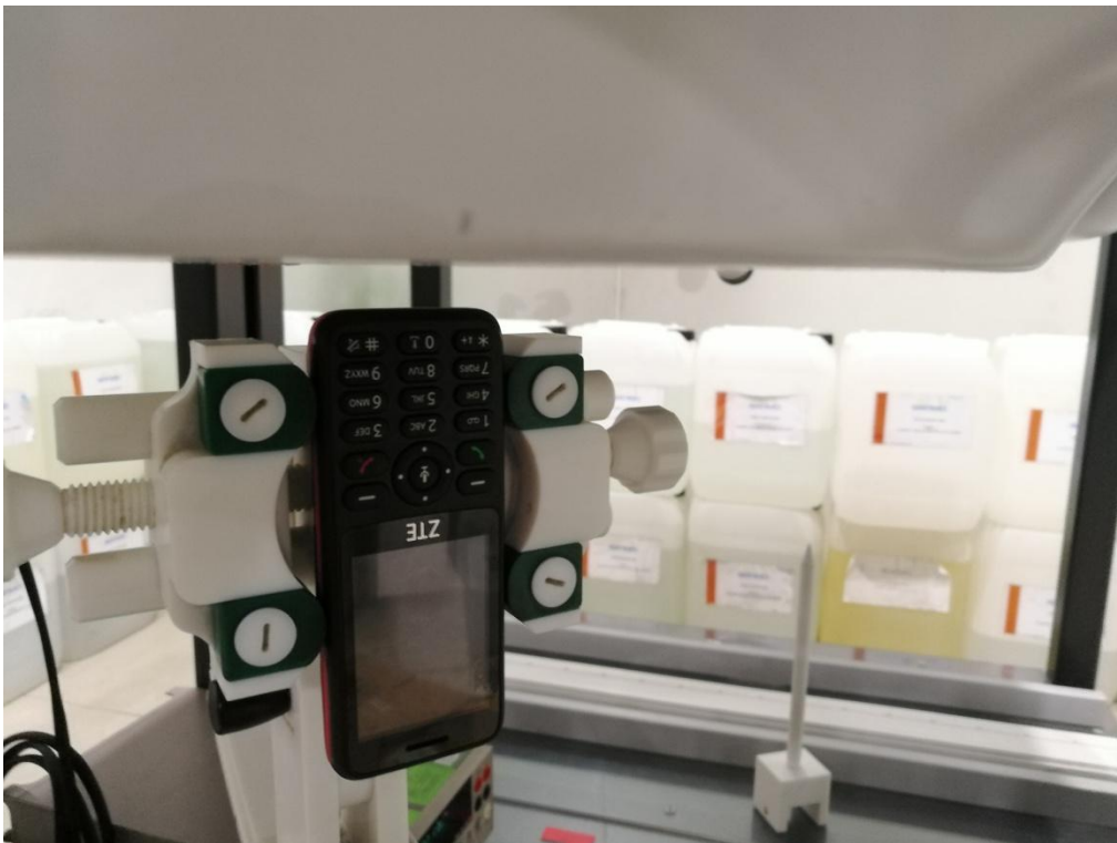
Body Bottom side(separation distance is 10mm)
