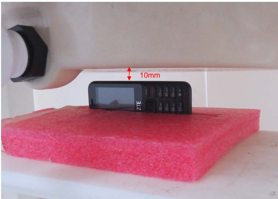
Picture 8: Right Side, the distance from handset to the bottom of the Phantom is 10mm
