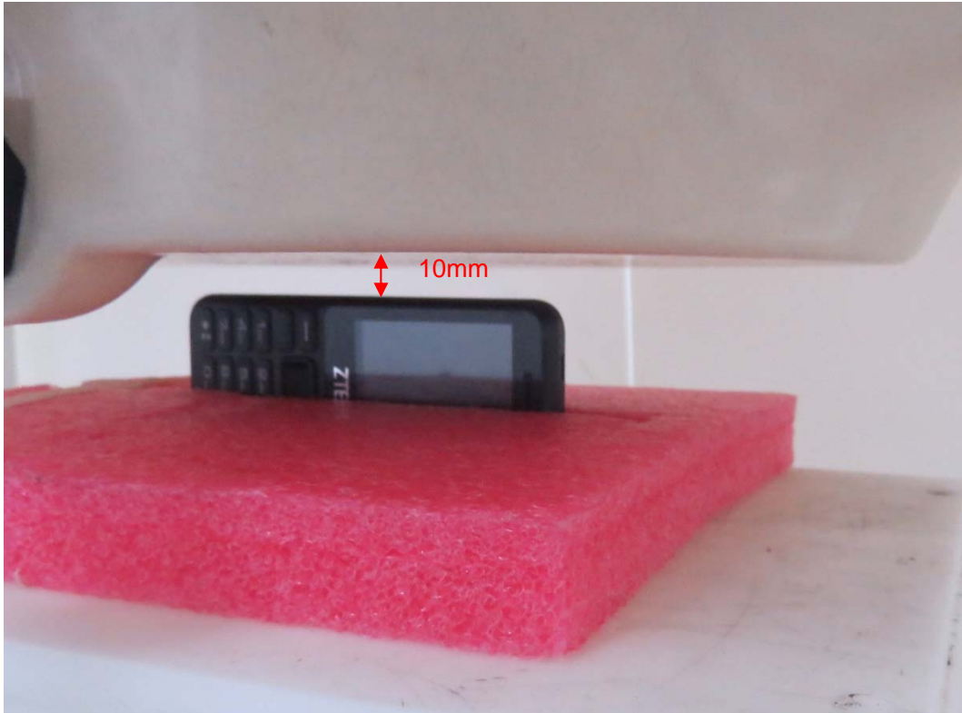
Picture 7: Left Side, the distance from handset to the bottom of the Phantom is 10mm
