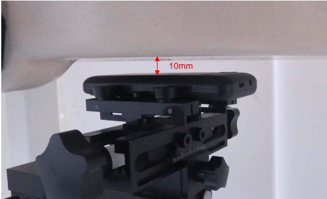
Picture 5: Back Side, the distance from handset to the bottom of the Phantom is 10mm
