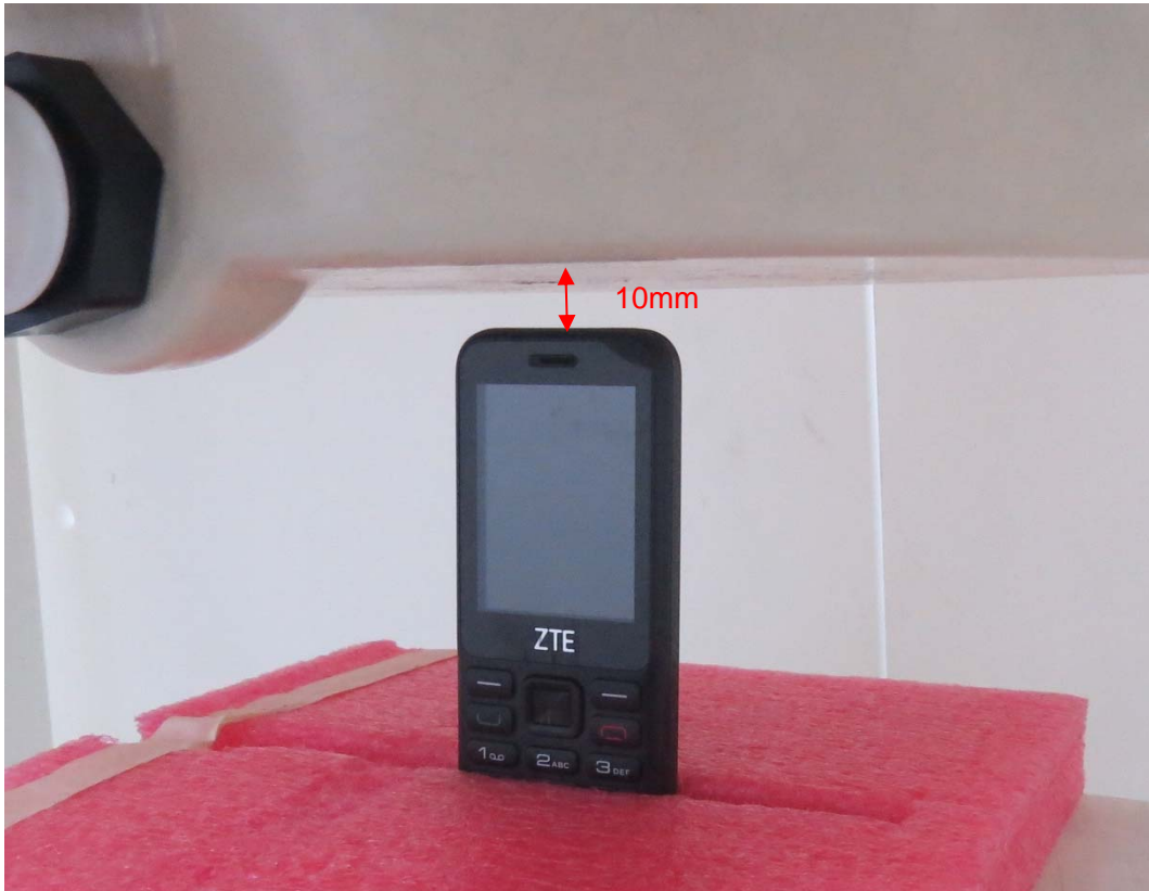
Picture 9: Top Side, the distance from handset to the bottom of the Phantom is 10mm
