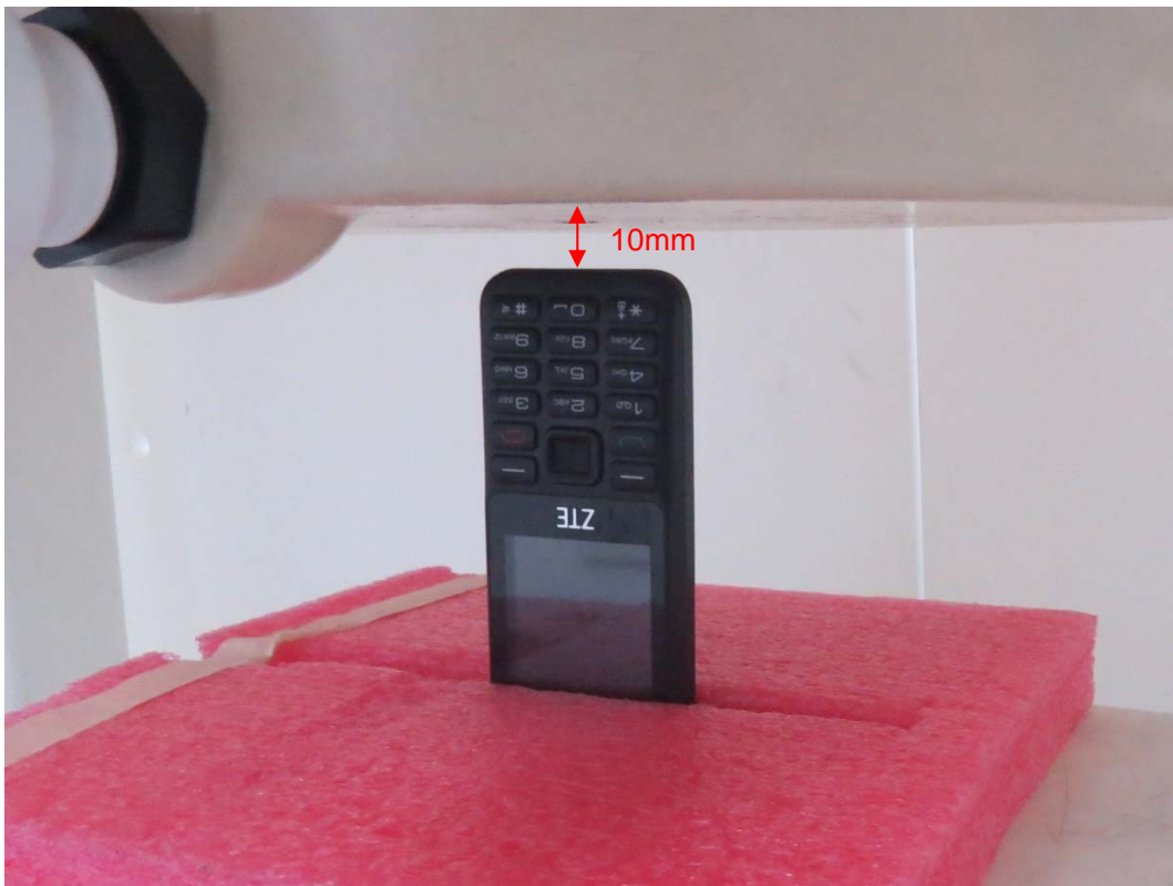
Picture 10: Bottom Side, the distance from handset to the bottom of the Phantom is 10mm
