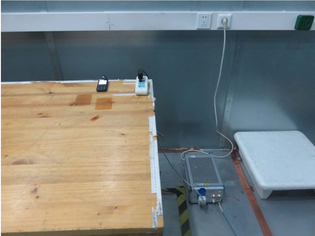
Picture 3 Conducted Emission Test Setup
