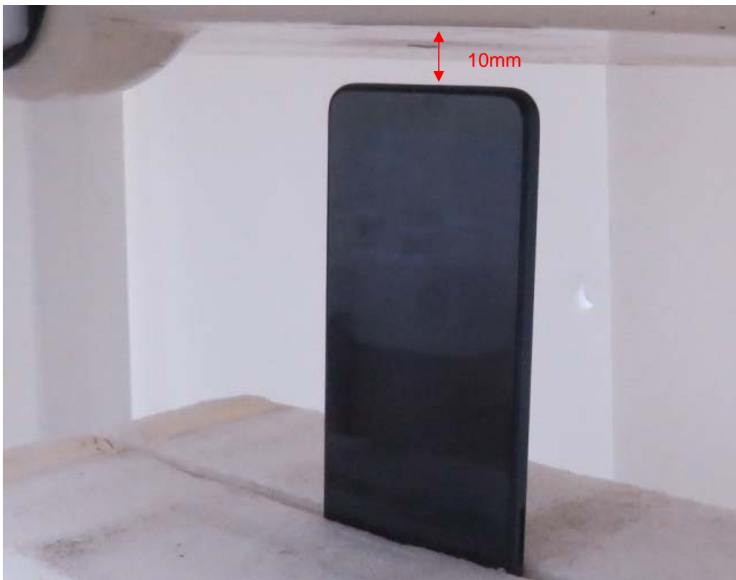
Picture 12: Bottom Edge, the distance from handset to the bottom of the Phantom is 10mm
