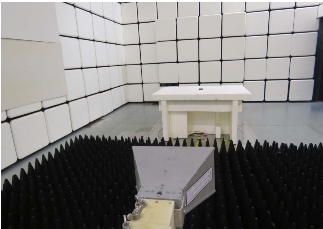
Picture 1: Radiated Spurious Emissions Test setup
