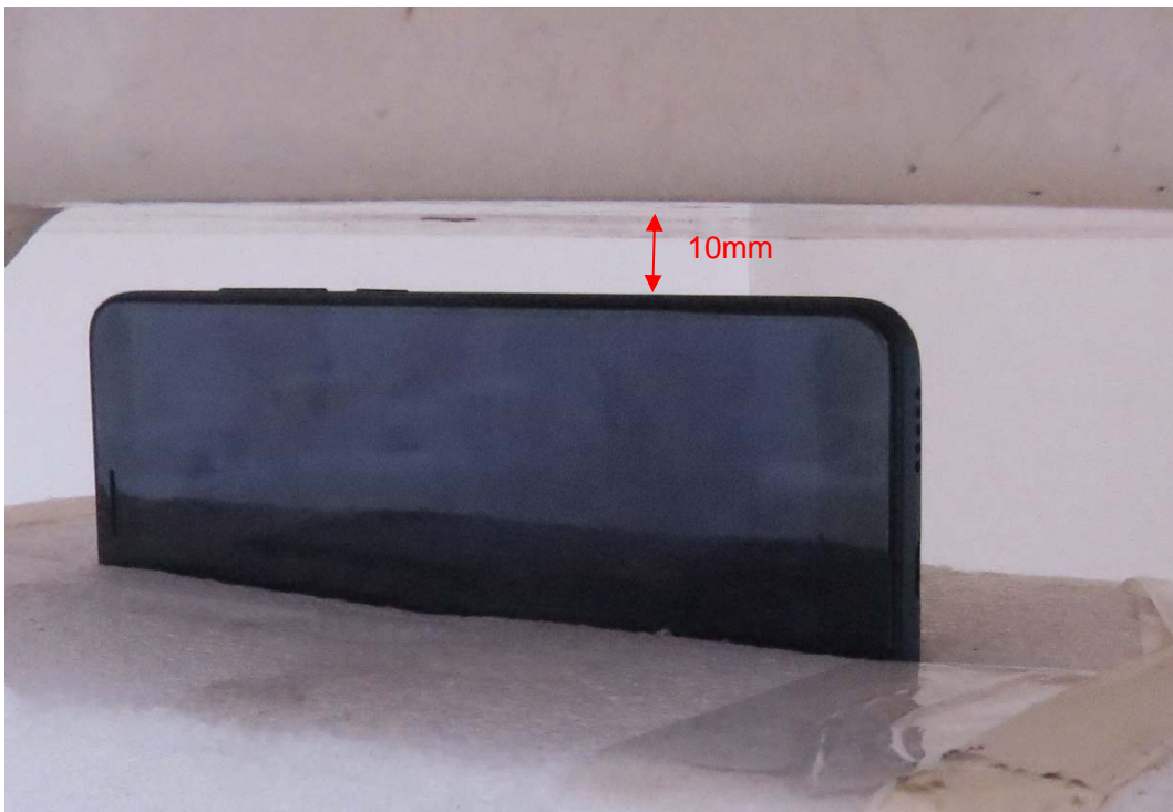
Picture 10: Right Side, the distance from handset to the bottom of the Phantom is 10mm
