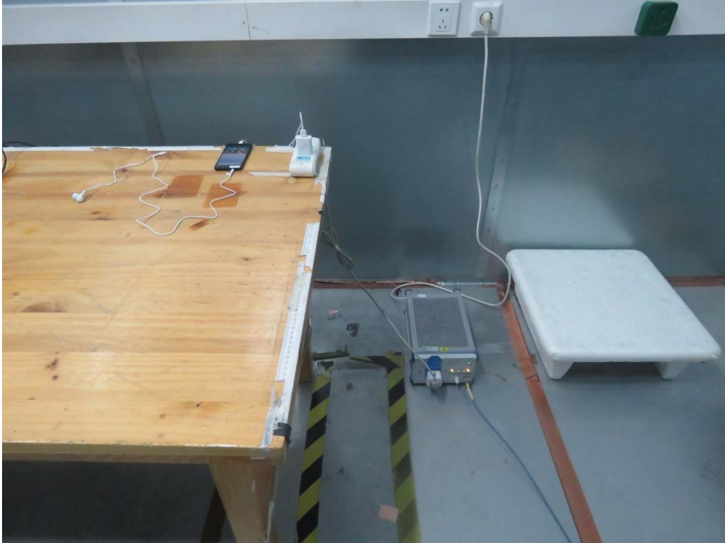
Picture 2 Conducted Emission Test Setup
