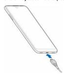
If the battery charge is low you may be unable to power on the phone. Leave on charge for at least 20 minutes and try again. Contact the customer service if you still cannot power on the phone after prolonged charging.
