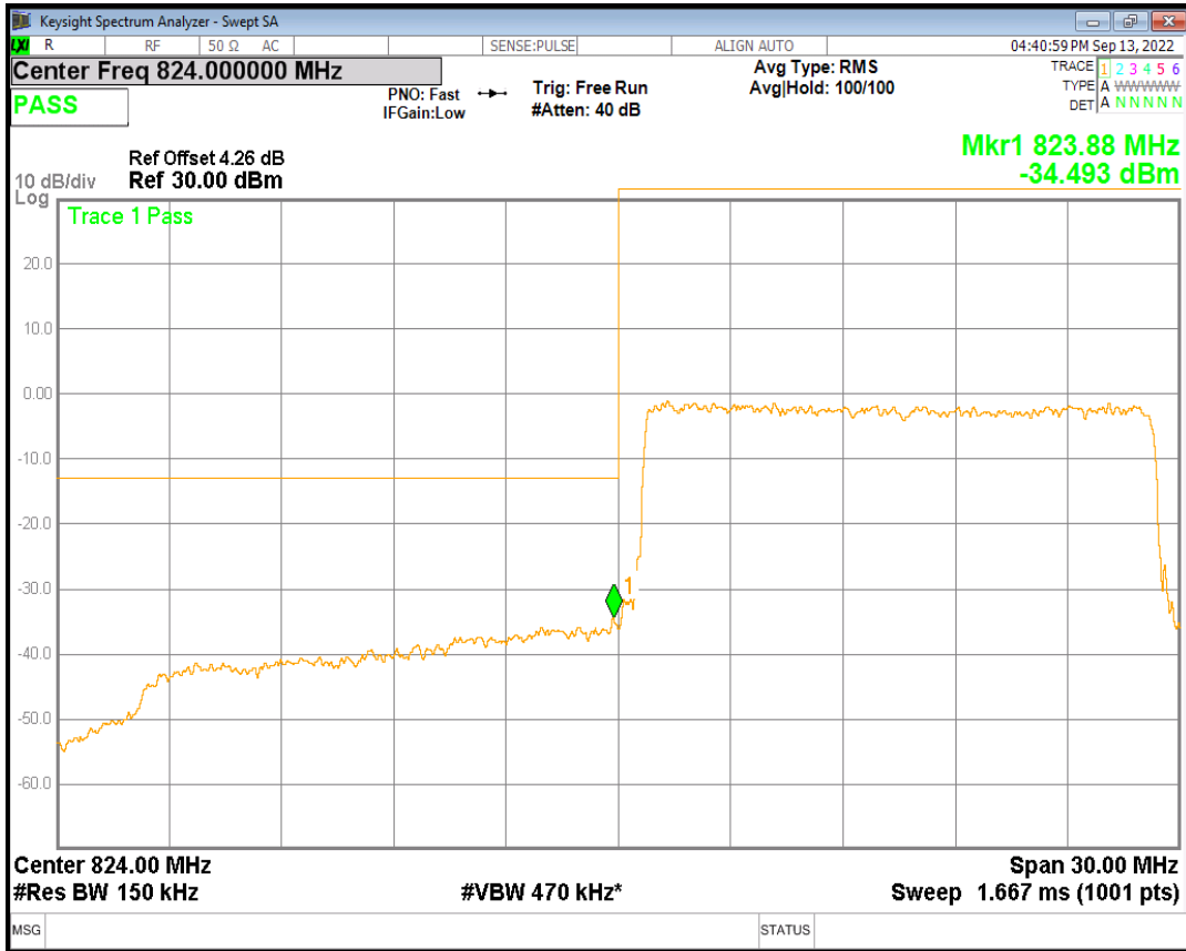
Band26(824-849) QPSK BW=15MHz Channel=26965 RB Size=75 Position=#0
