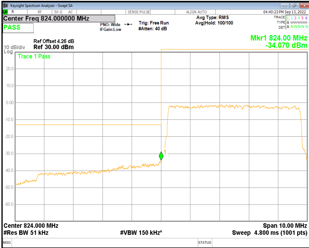
Band26(824-849) QPSK BW=5MHz Channel=27015 RB Size=25 Position=#0
