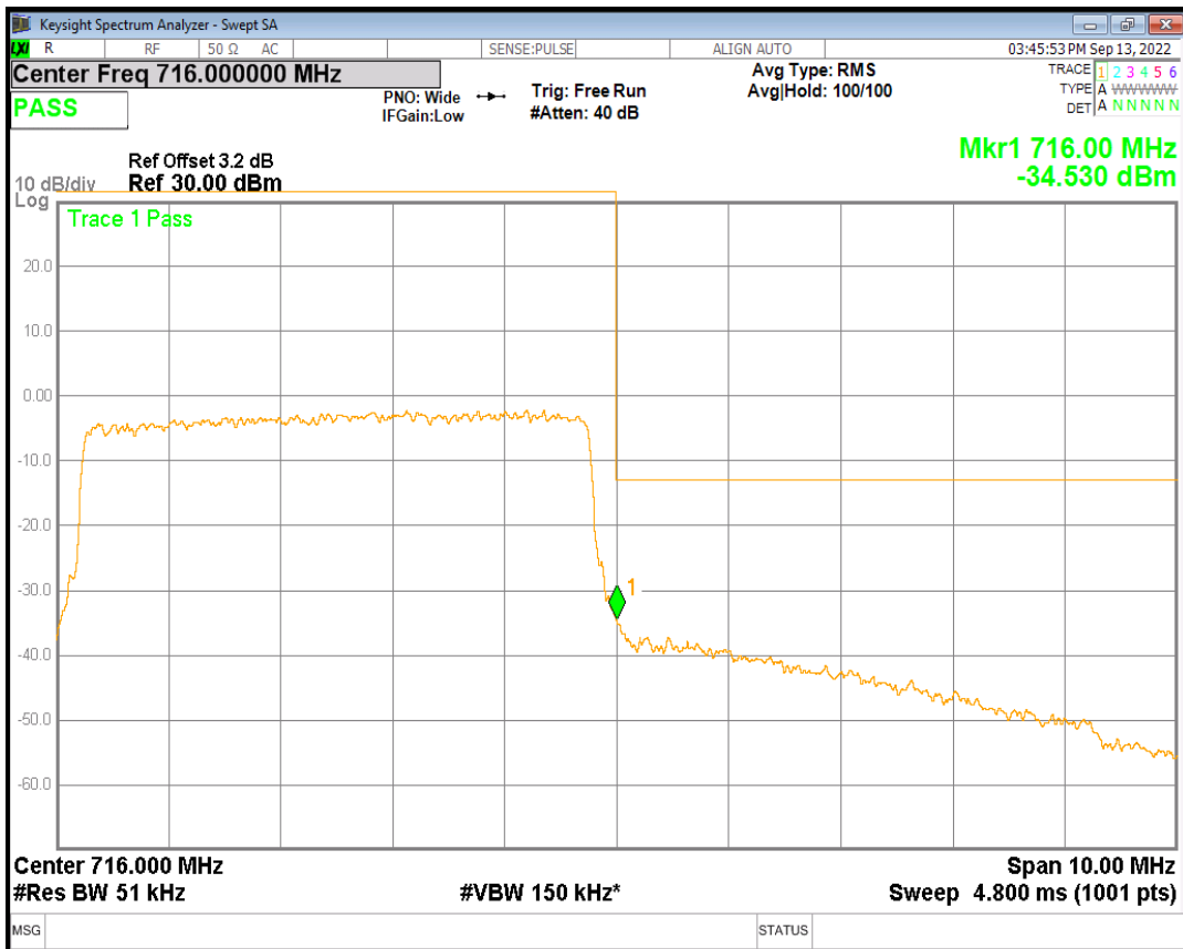
Band2 QAM16 BW=1.4MHz Channel=18607 RB Size=6 Position=#0
