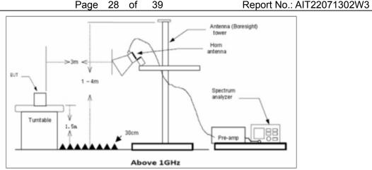
Above 18 GHz shall be extrapolated to the specified distance using an extrapolation factor of 20 dB/decade form 3m to 1m.
