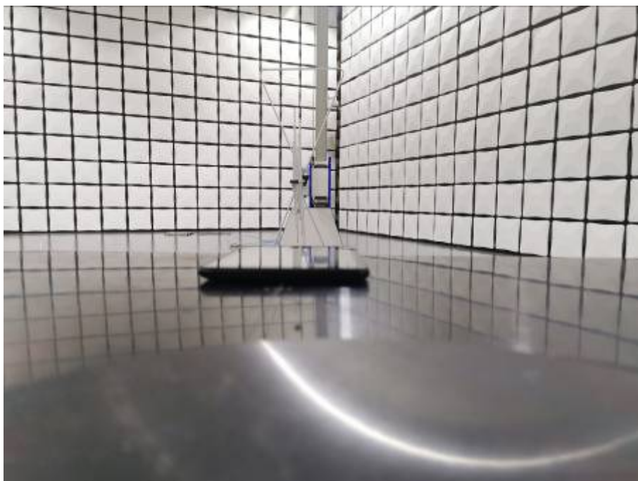
Radiated Emissions Test Setup (with charger) (30-1000MHz)
