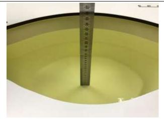
Liquid depth in the Head phantom
