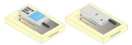
Picture 4 Test positions for body-worn devices
