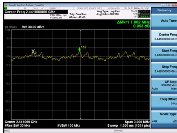
BT 3DH5 CH39, Carrier frequency (MHz): 2441
