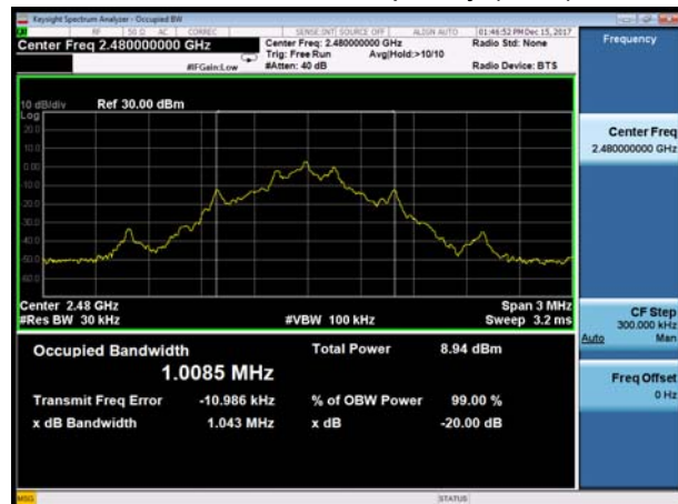
BT DH5 CH78, Carrier frequency (MHz): 2480
