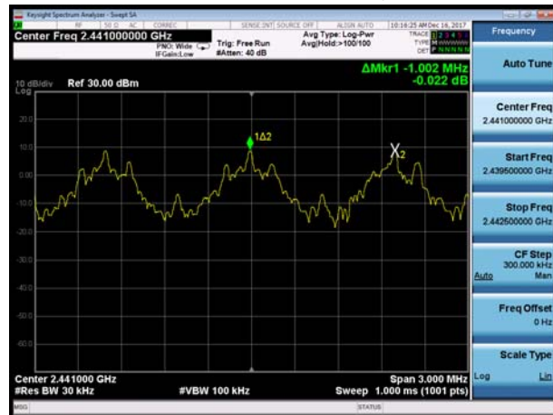
BT 3DH5 CH39, Carrier frequency (MHz): 2441
