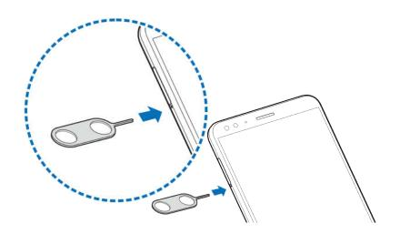
Pull out the card tray and place the nano-SIM card (right)
