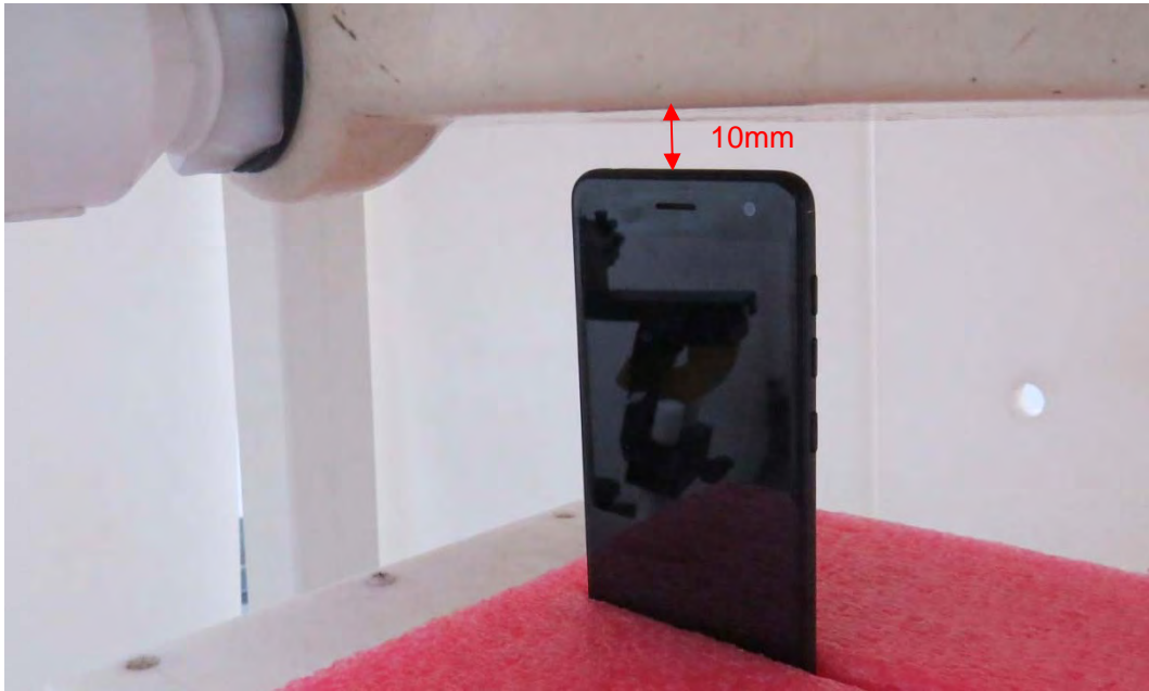
Picture 26: Top Side, the distance from handset to the bottom of the Phantom is 10mm
