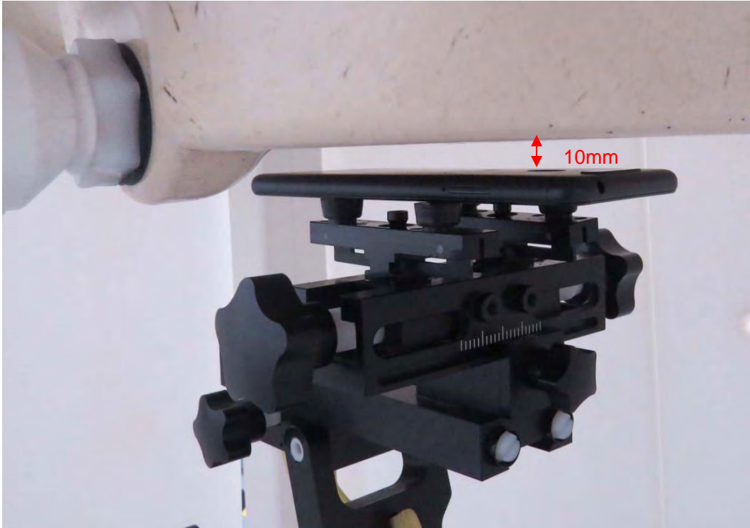
Picture 20: Back Side, the distance from handset to the bottom of the Phantom is 10mm
