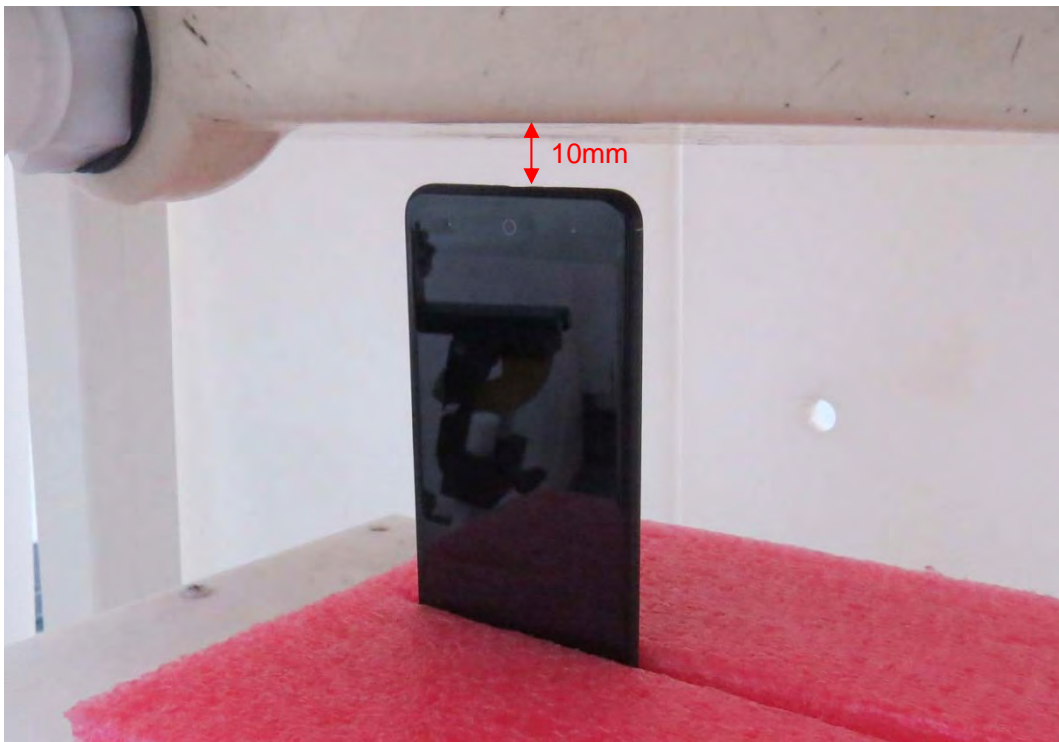
Picture 27: Bottom Side, the distance from handset to the bottom of the Phantom is 10mm
