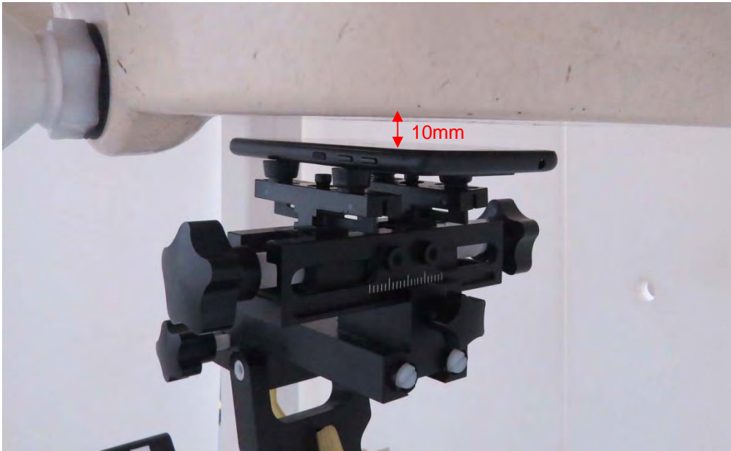
Picture 22: Front Side, the distance from handset to the bottom of the Phantom is 10mm
