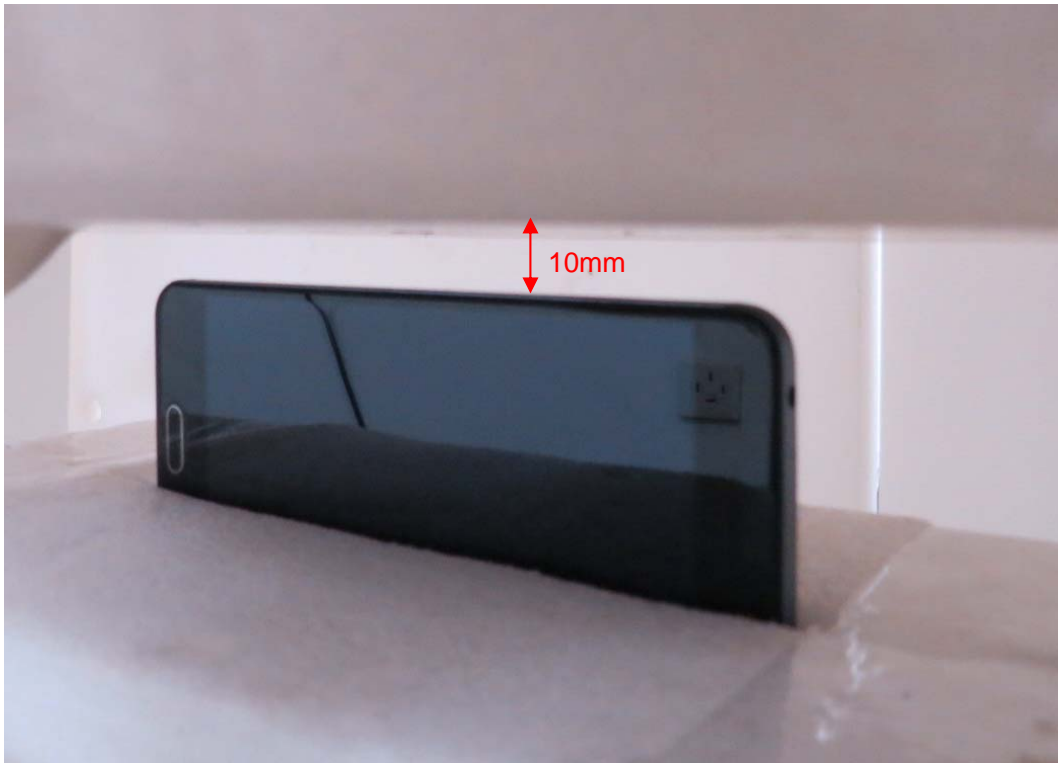
Left Side, the distance from handset to the bottom of the Phantom is 10mm
