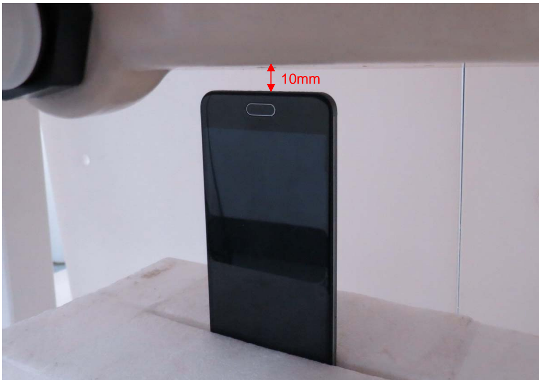
Bottom Side, the distance from handset to the bottom of the Phantom is 10mm
