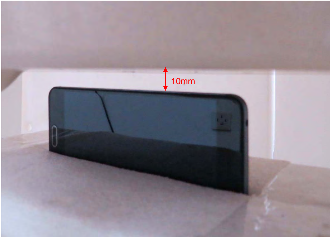
Picture 20: Left Side, the distance from handset to the bottom of the Phantom is 10mm
