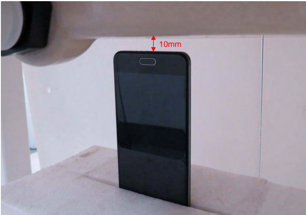
Picture 23: Bottom Side, the distance from handset to the bottom of the Phantom is 10mm
