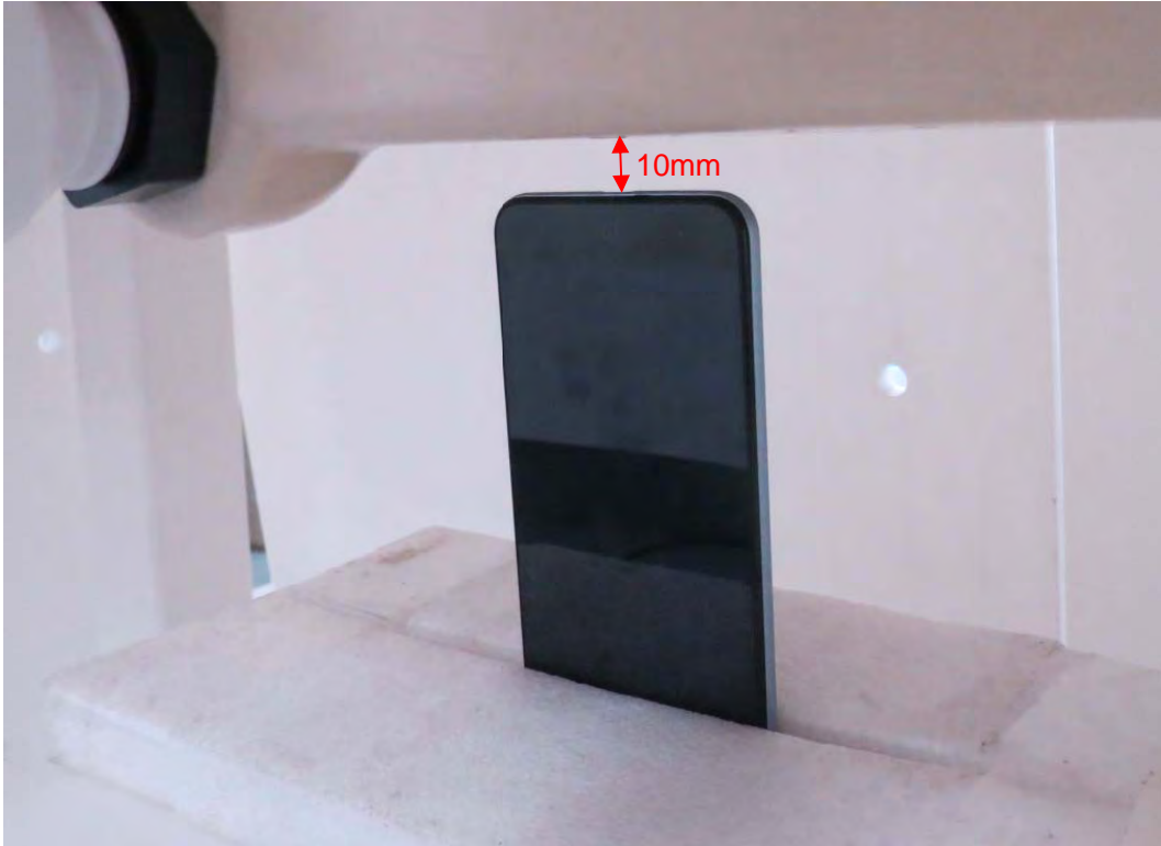
Picture 22: Top Side, the distance from handset to the bottom of the Phantom is 10mm
